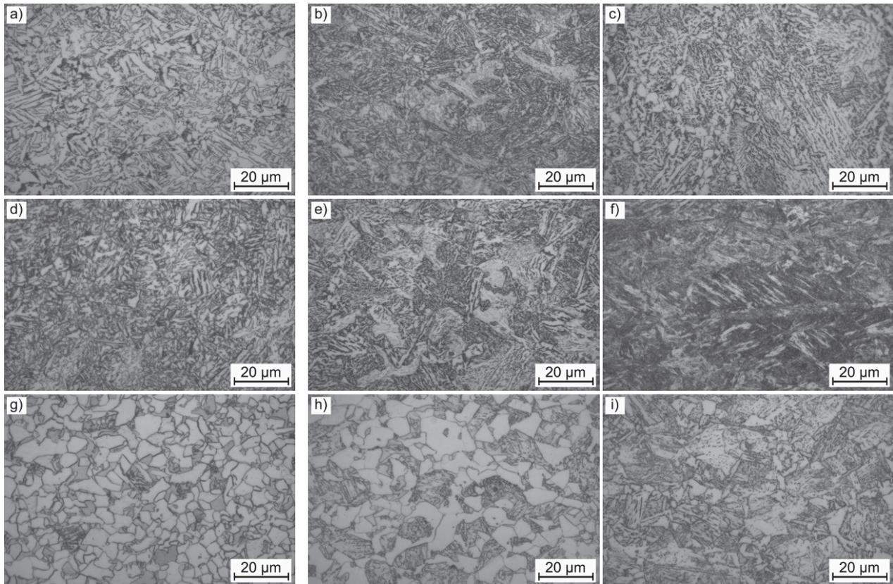
**Figure 4** Microstructure of forged and direct-cooled laboratory samples: a) - c) steel A, d)-f) steel B, g)-i) steel C, for treatments: a),d),g) - cycle 1, b),e),h) - cycle 2, and c),f),i) - cycle 3; etched in 5 % nital
