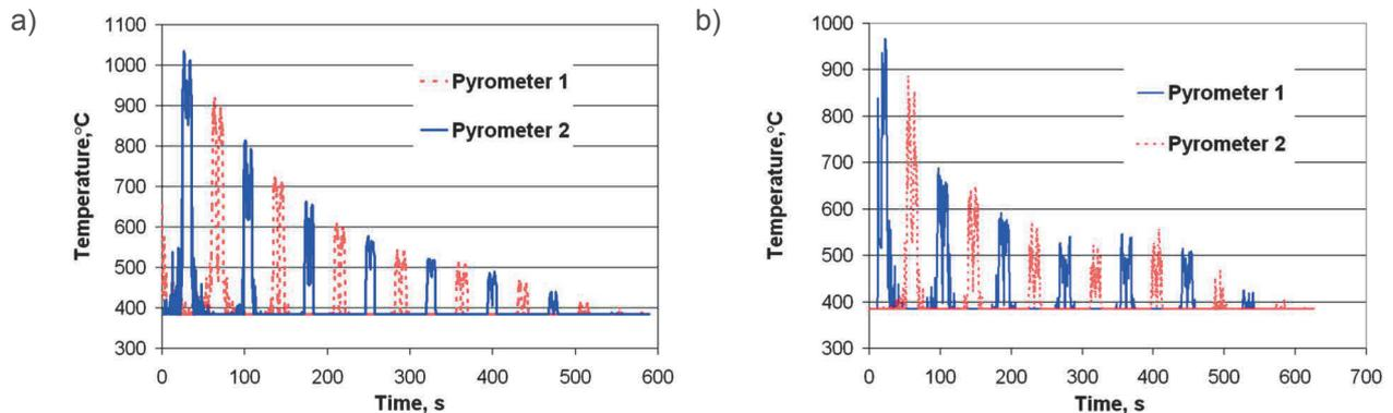
**Figure 3** Cooling curves plotted by surface temperature in semi-industrial modeling: a) cycle 1, b) cycle 2
