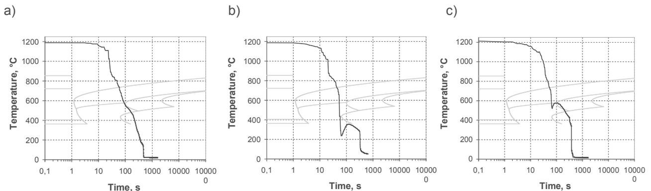
**Figure 2** Experimental temperature plots recorded for: a) cycle 1, b-c) cycles 2 and 3, respectively, on the background of CTT diagram of Steel 3
