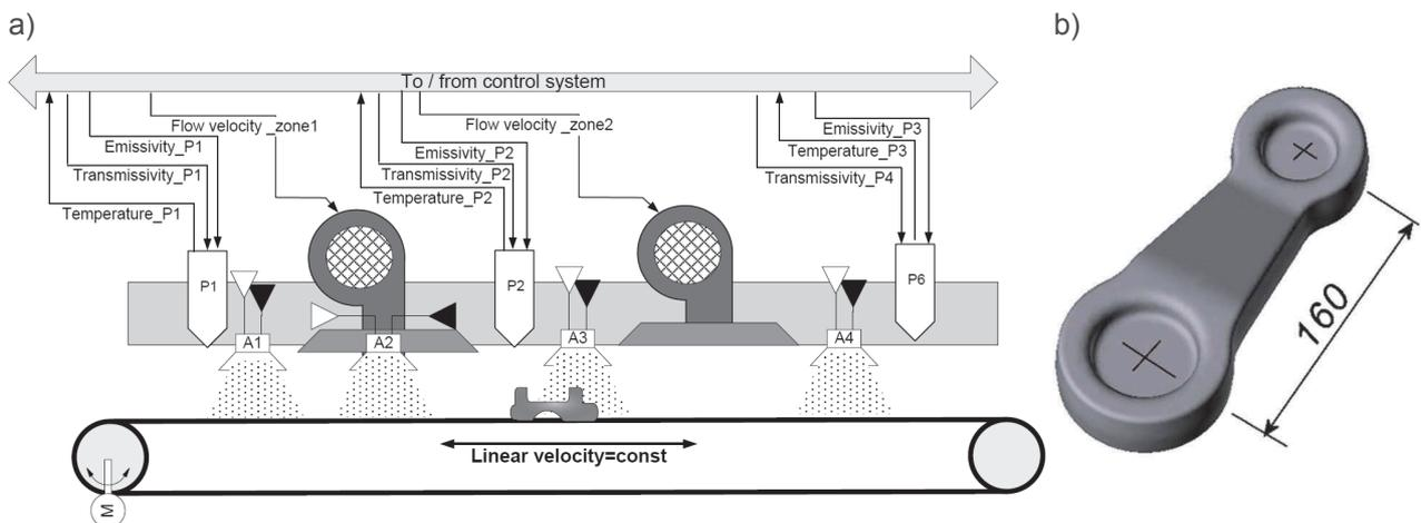
**Figure 1** Scheme of the semi-industrial cooling simulator (a), and geometry of specimens: b) geometry of the sample used for industrial verification
