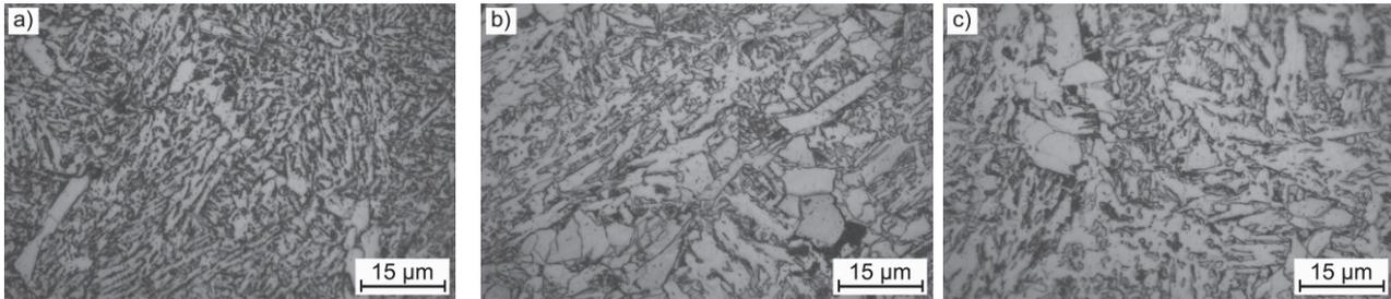
**Figure 5** Microstructure in the core of the forged part from Figure 1b obtained for: a) steel A, b) steel B, c) steel C, after austempering (cycle 2) in semi-industrial conditions; etched in 5 % nital
