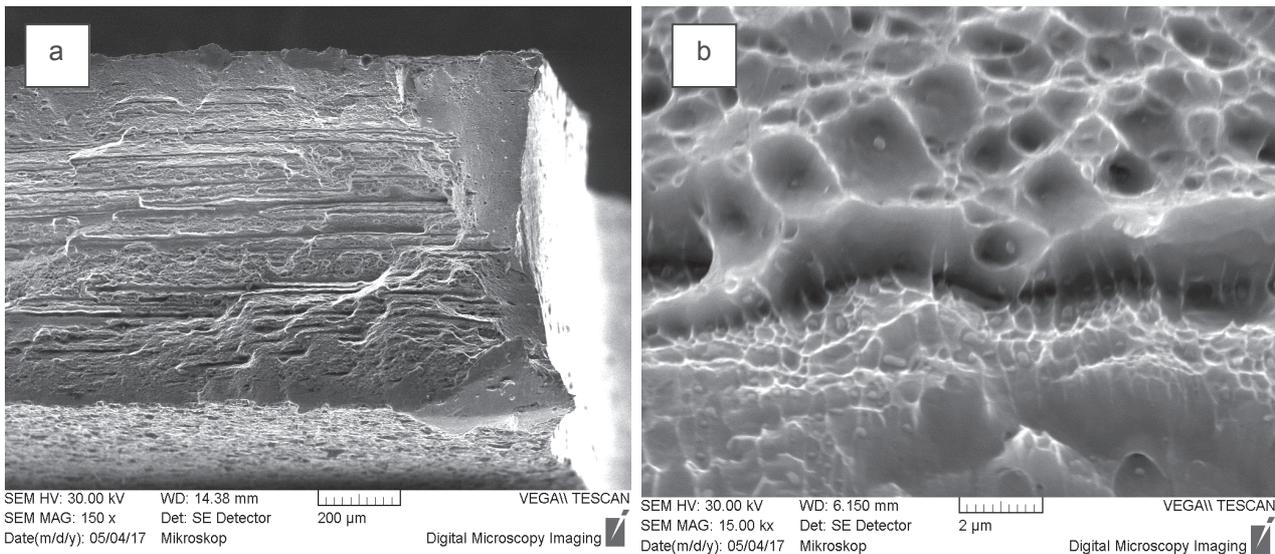
**Figure 3 (a)** Defective fracture mode due to precipitation
