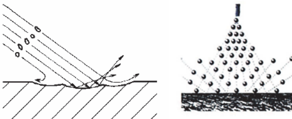
Figure 2 Abrasive - Erosion / Impact wear, shot blasting principle [5]
