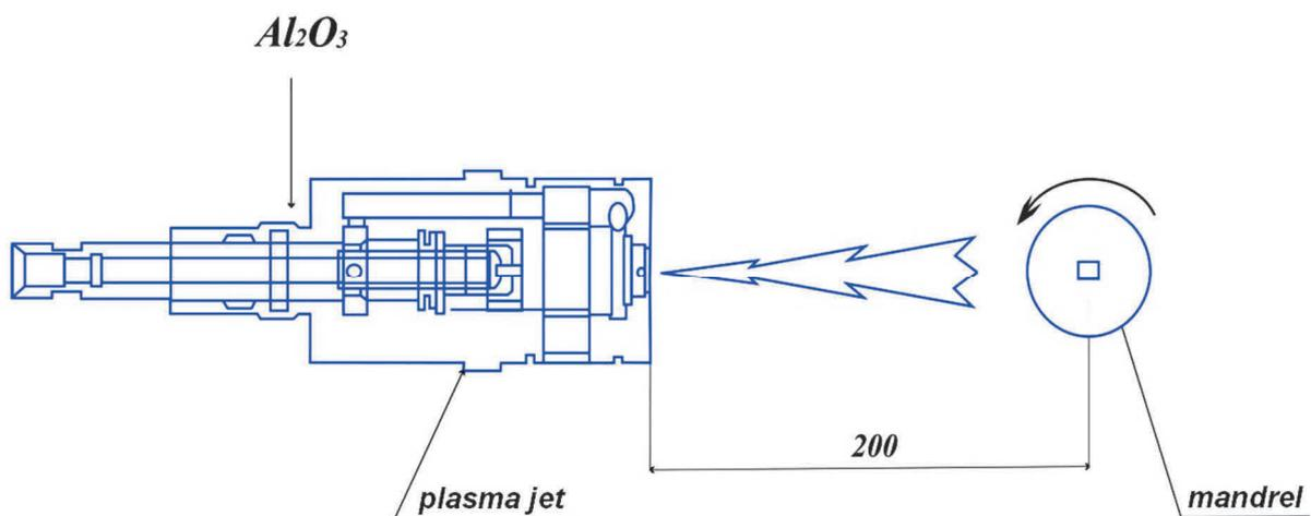
**Figure 2** The scheme of spray deposition
