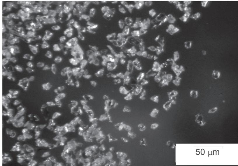
**Figure 1** Optical image of alumina powder used for plasma spray deposition ( $\times 200$ )
