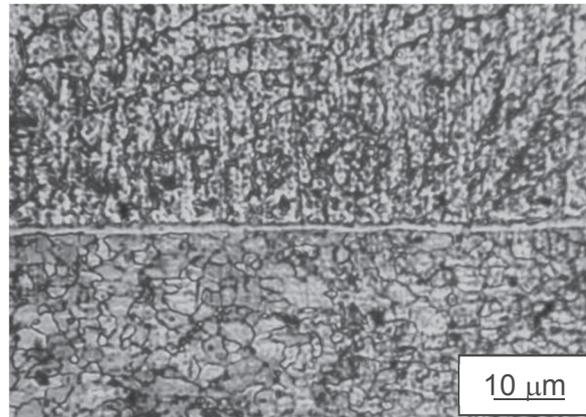
**Figure 5** Galvanized steel interface microstructure - Al alloy (2 % NiAl)
