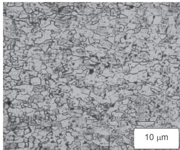
**Figure 4** Galvanized steel microstructure
