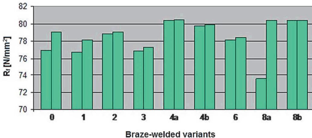
**Figure 7** The histogram of shear strength values
