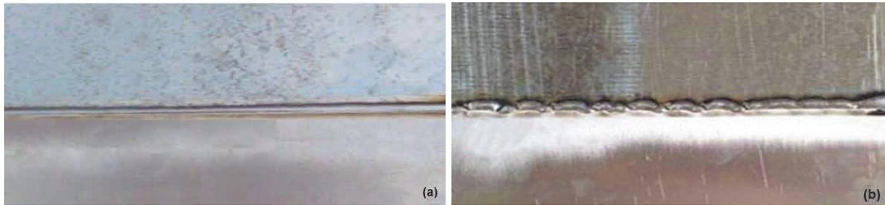
**Figure 1** The visual appearance of the surface of braze-welded joints:
