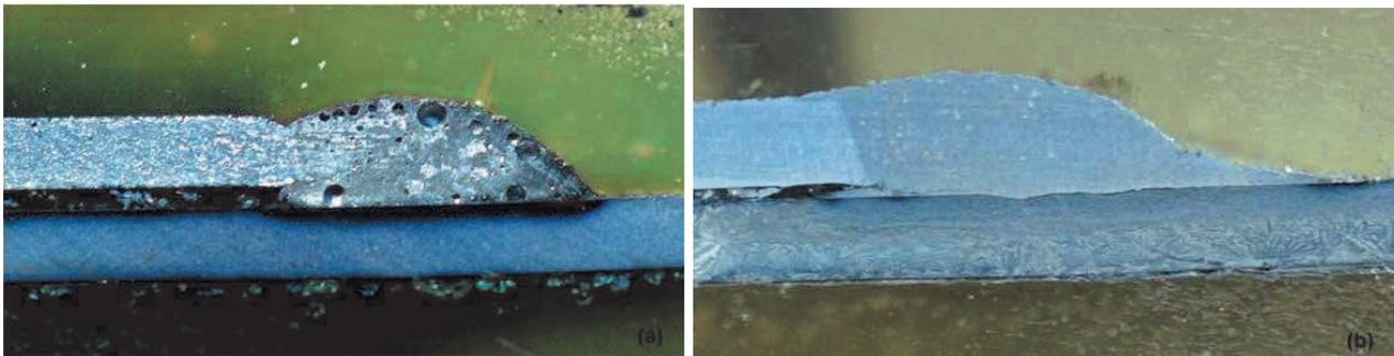
**Figure 2** Macrographic image of the cross section of braze-welded joints:
