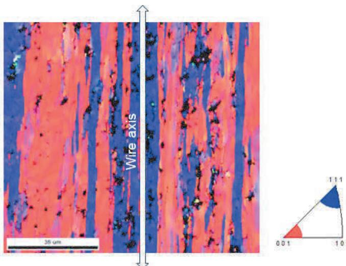
**Figure 2** Microstructure characterized by EBSD of the center of the 86 % deformed wire. Crystallographic directions parallel to the wire axis
