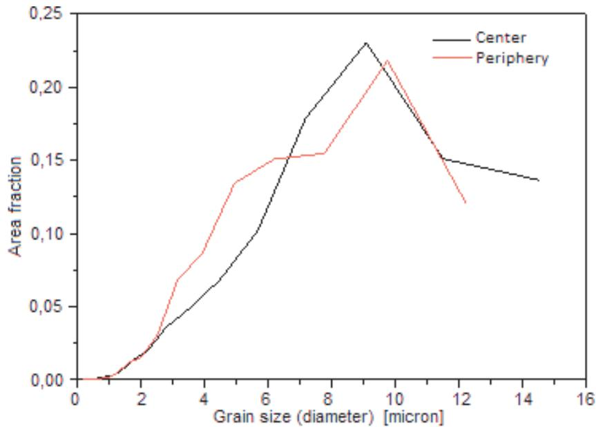
**Figure 5** Distribution of the grain size at the center and the periphery of the 86 % deformed wire annealed at 400 °C for 10 minutes
