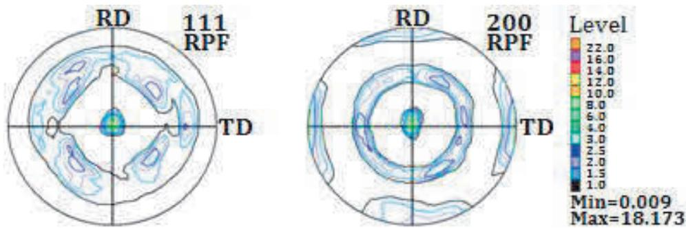
**Figure 1** Pole figures of the initial state (wire rod). ND is the wire axis, normal to the pole figures.
