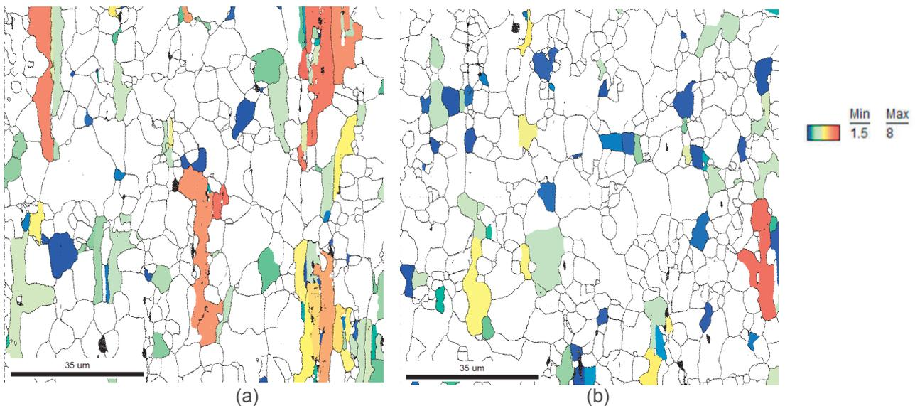
**Figure 8** (a): center; (b): periphery; in color, grains with GOS>1.5°, = non-recrystallized grains after 10 minutes at 400 °C
