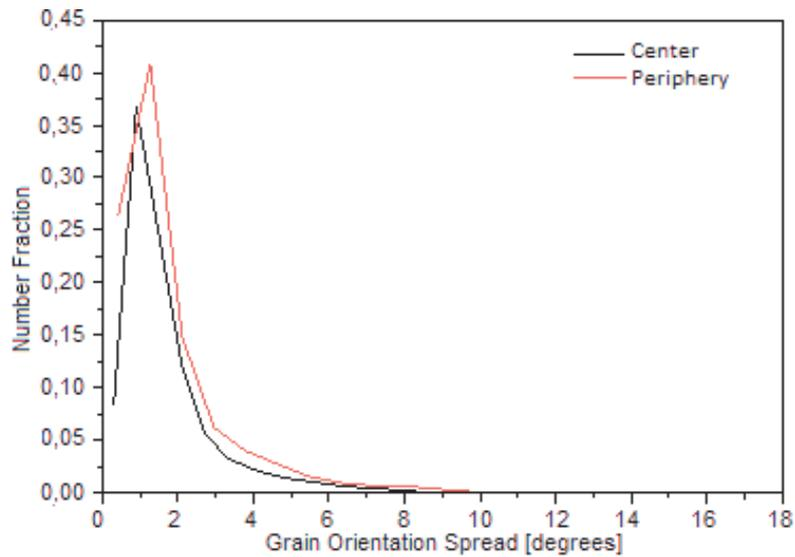
**Figure 7** GOS through the wire cross section after 10 minutes at 400 °C
