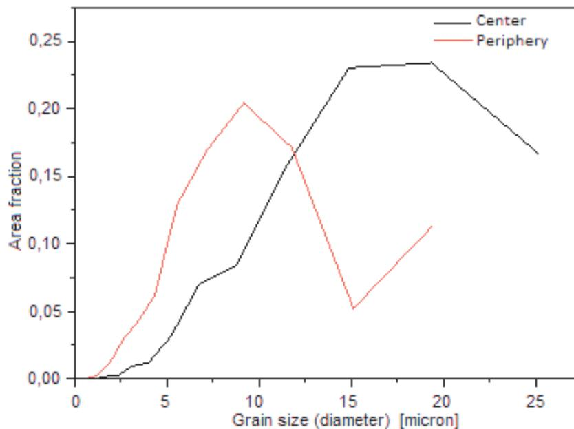
**Figure 6** Distribution of the grain size at the center and the periphery of the 86 % deformed wire annealed at 400 °C for 30 minutes
