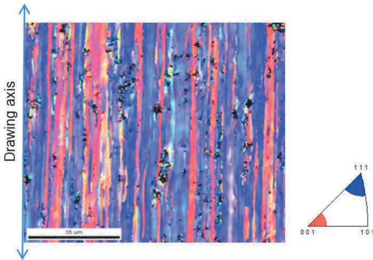
**Figure 3** Microstructure characterized by EBSD of the periphery of the 86 % deformed wire. Crystallographic directions parallel to the wire axis
