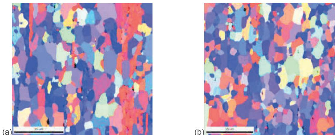
**Figure 4** Microstructures characterized by EBSD at the center (a) and at the periphery (b) of the 86 % deformed wire annealed at 400 °C for 10 minutes
