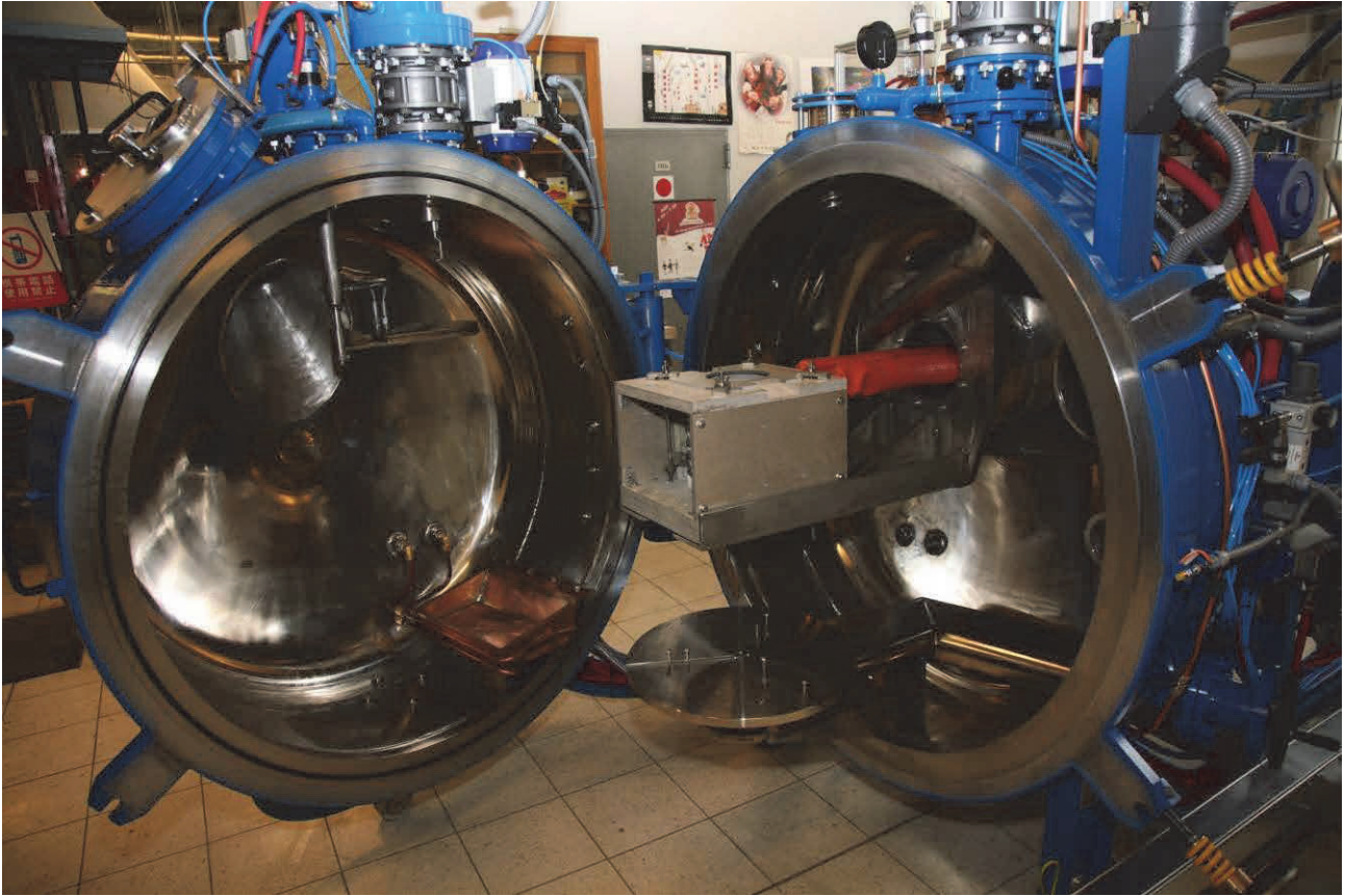
Figure 3 The laboratory vacuum furnace with a capacity of 10 kg
