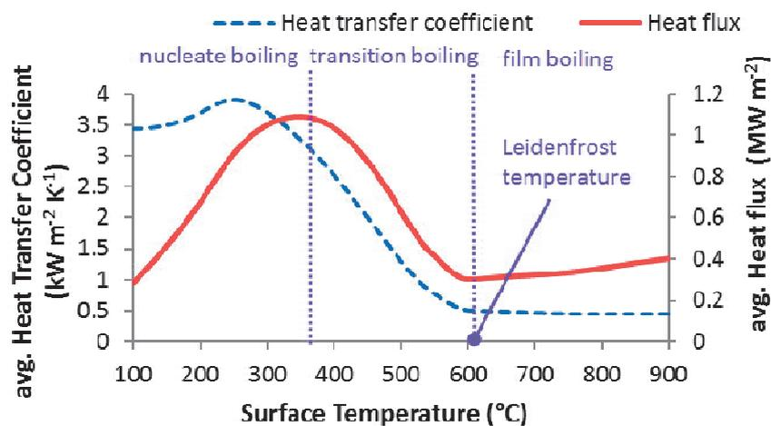
**Figure 3** Dependences of the heat transfer coefficient (blue) and heat flux (red) on the surface temperature
