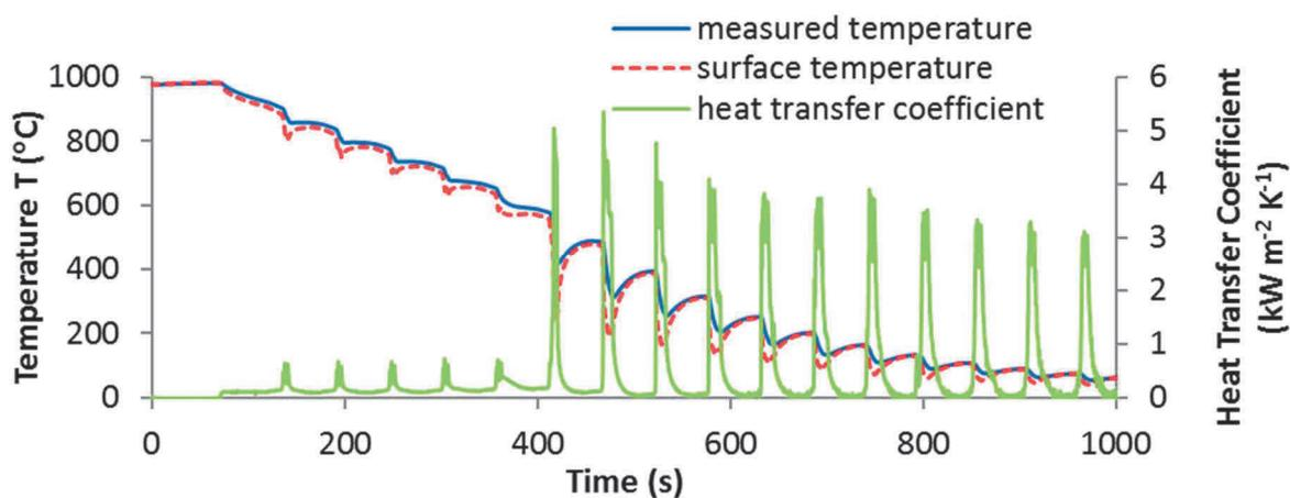
**Figure 2** Measured temperature, computed surface temperature, and computed heat transfer coefficient
