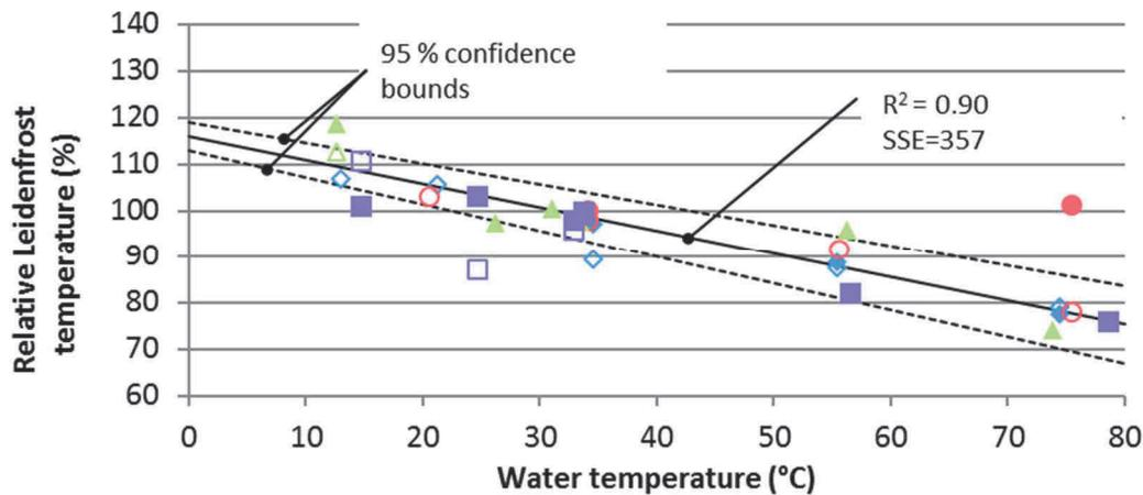
**Figure 7** Influence of the water temperature on the Leidenfrost temperature
