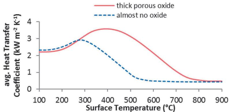
**Figure 5** Influence of the oxide layer on the heat transfer coefficient [12]
