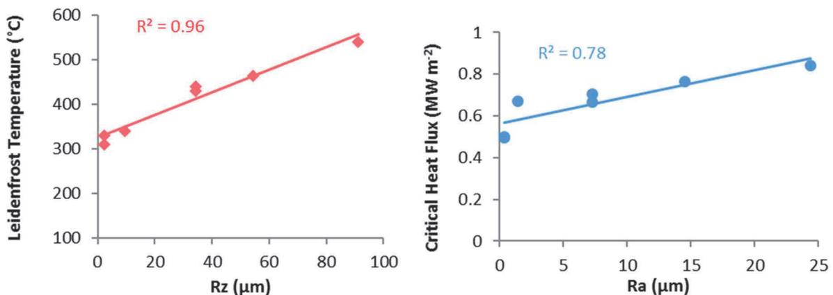
**Figure 4** Dependence of the critical heat flux on the surface roughness parameter Ra (left) and dependence of the Leidenfrost temperature on the surface roughness parameter Rz (right) [8]
