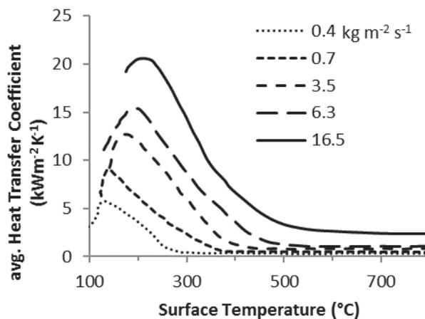
**Figure 6** Influence of the water impact density on the heat transfer coefficient [14]
