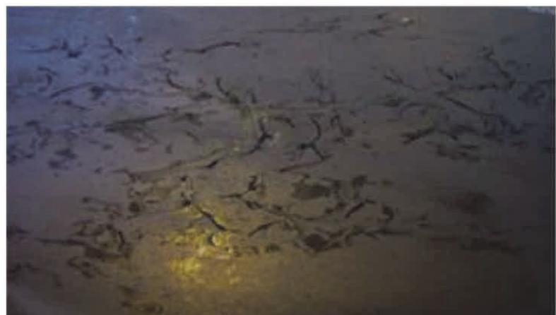
**Figure 3** Typical star crack defect
