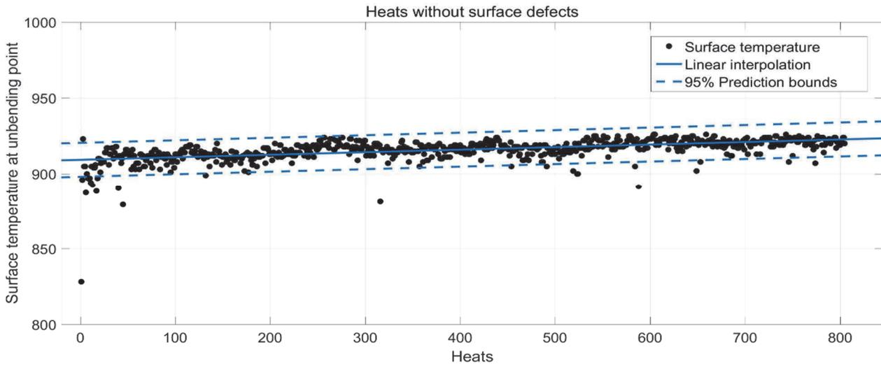
**Figure 4** Surface temperatures with 95 % prediction bounds (without defects)
