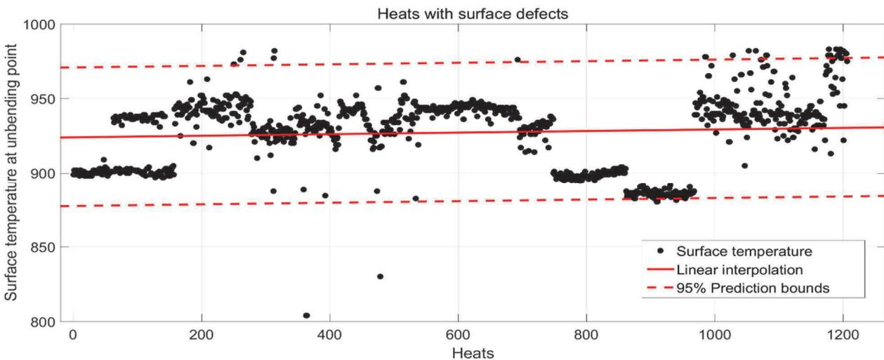
**Figure 5** Surface temperatures with 95 % prediction bounds (with defects)
