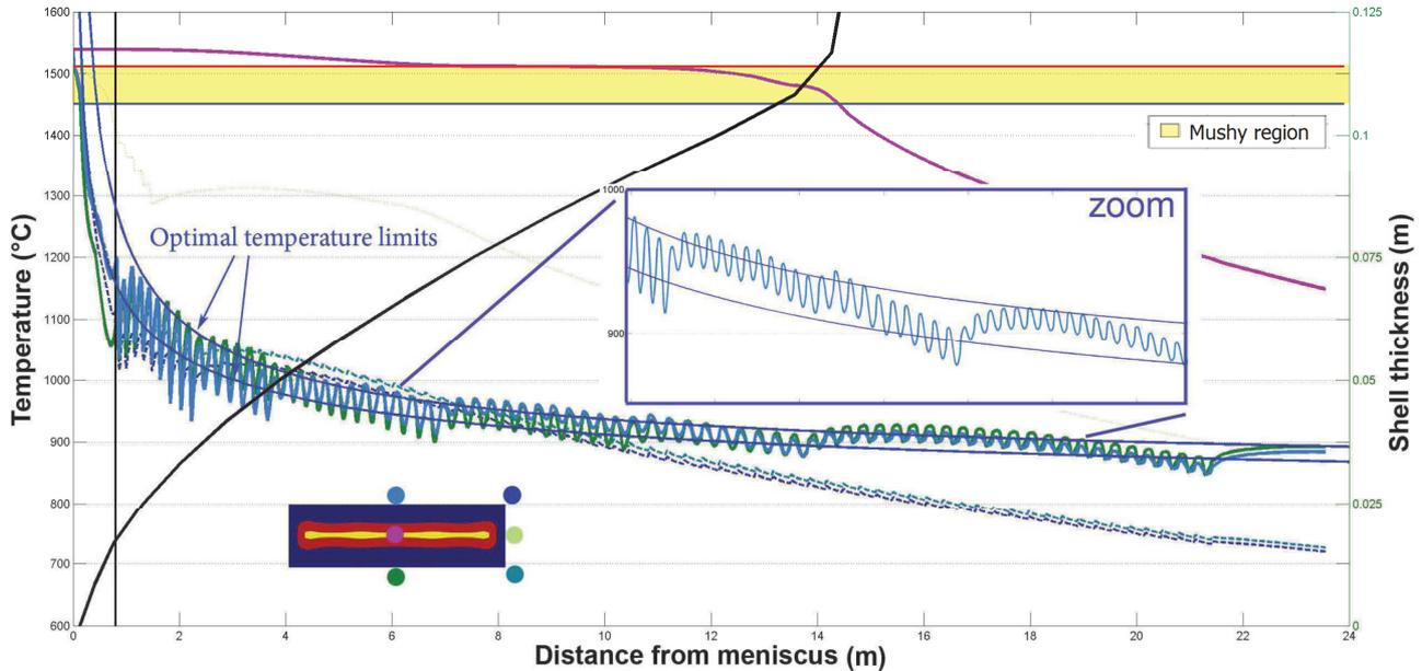
**Figure 6** Optimal temperature field
