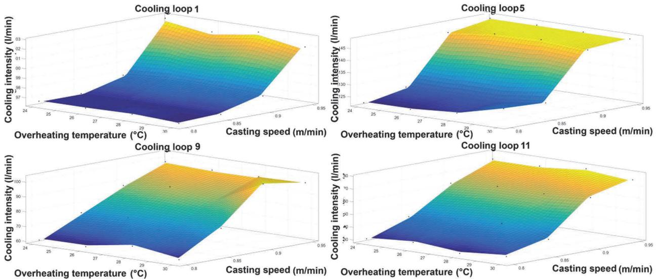
**Figure 7** Optimal cooling intensity for four particular cooling loops
