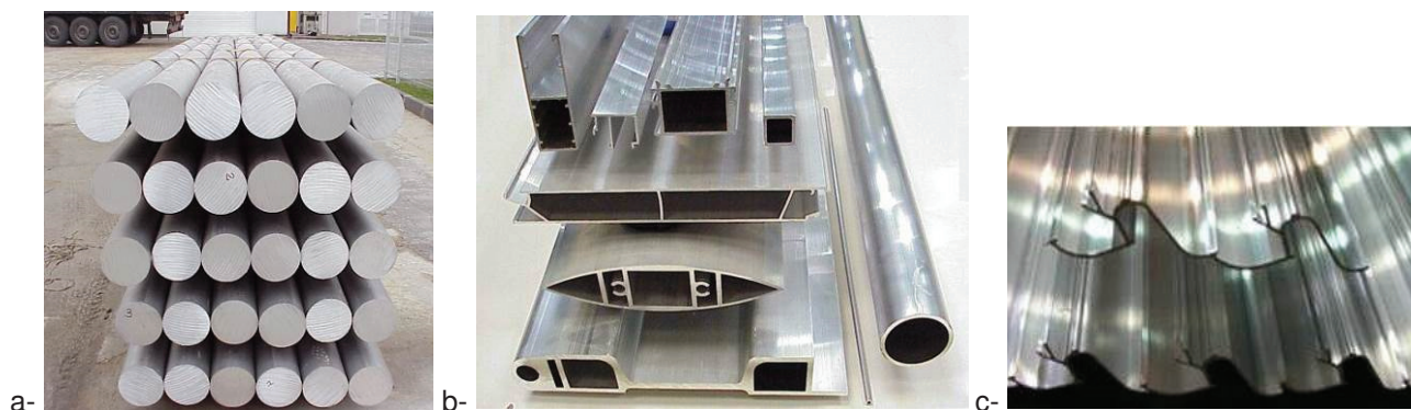
Figure 4 Examples of the product realized in the production of: a) raw materials batch, b) the finished product - hollow sections, c) the finished product - open profiles
