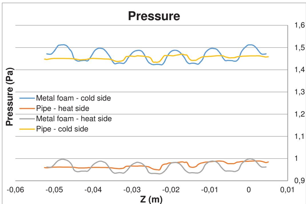
**Figure 8** Pressure distribution in heat exchangers
