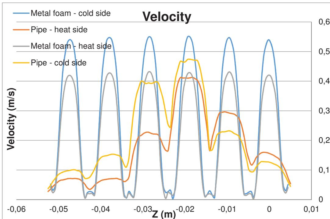
**Figure 6** Velocity profile of the heat exchangers
