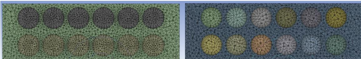
**Figure 3** From left: Computing meshes of the metal foams and tube heat exchanger
