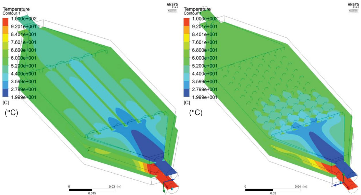
Figure 10 Cold side of the heat exchangers
