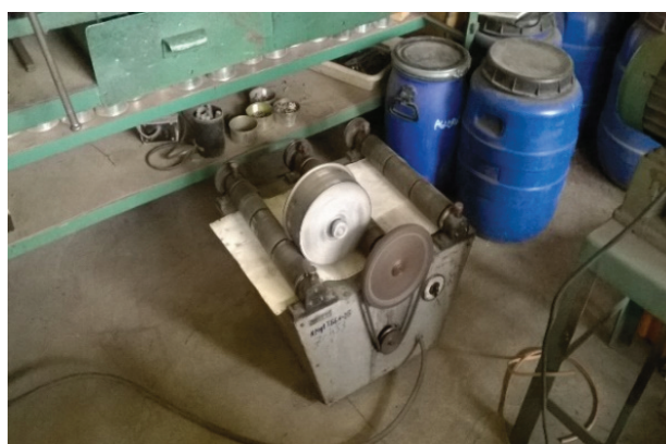
Figure 2 The laboratory roller mill
