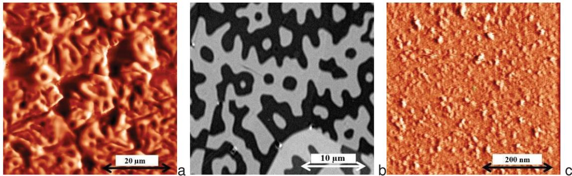
**Figure 2** Domain structure on the pole surface of PM2 magnet: (a) magnetic AFM and (b) magneto-optic Kerr effect; (c) AFM image of the pole surface of PM2 magnet after electrochemical etching
