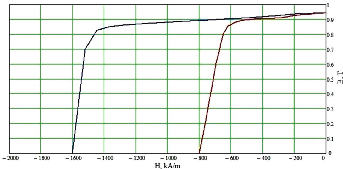
**Figure 1** Magnetization reversal curves for permanent magnets (red curve) PM1 and (blue curve) PM2
