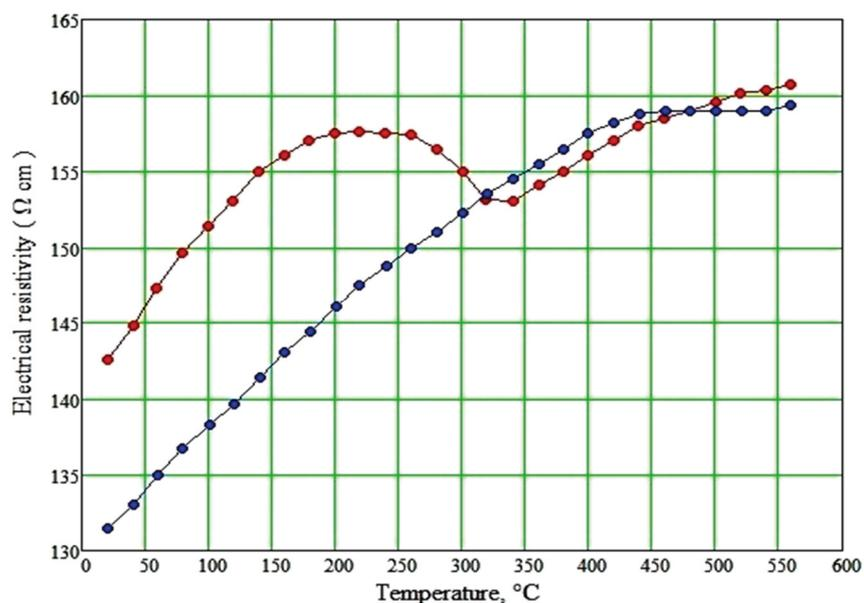
**Figure 3** Temperature dependences of the electrical resistivity for magnet PM2 (blue curve) and reference cobalt-free magnet (red curve)
