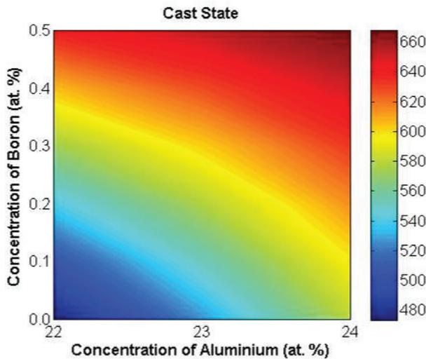
**Figure 8** A comparison of values of the yield strengths for the castings of the Ni-22Al, Ni-24Al, Ni-22Al-0.5B and Ni-24Al-0.5B alloys determined by compression tests at a temperature of 800 °C
