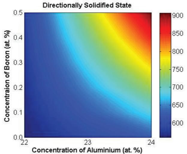
**Figure 9** A comparison of values of the yield strengths for the Ni-22Al, Ni-24Al, Ni-22Al-0.5B and Ni-24Al-0.5B alloys after directional solidification determined by compression tests at a temperature of 800 °C
