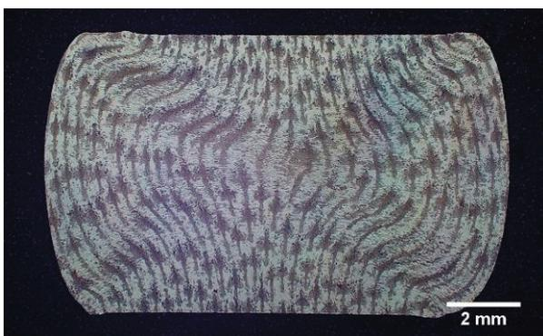
**Figure 5** The sample of the Ni-22Al-0.5B alloy in directionally solidified state after compression test
