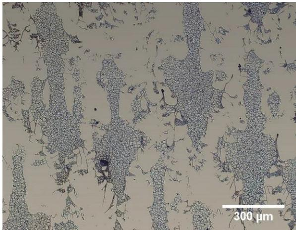
**Figure 1** A detail of the directionally solidified structure of the Ni-22Al-0.5B alloy
