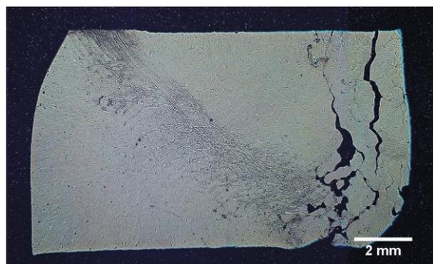
**Figure 6** The sample of the Ni-24Al-0.5B alloy in directionally solidified state after compression test
