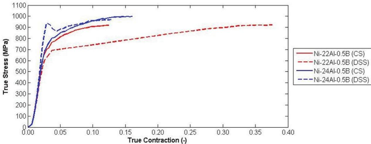
**Figure 7** A plot of the compression test processes carried out on the castings and directionally solidified samples of the Ni-22Al-0.5B and Ni24Al-0.5B alloys at the temperature of 800 °C
