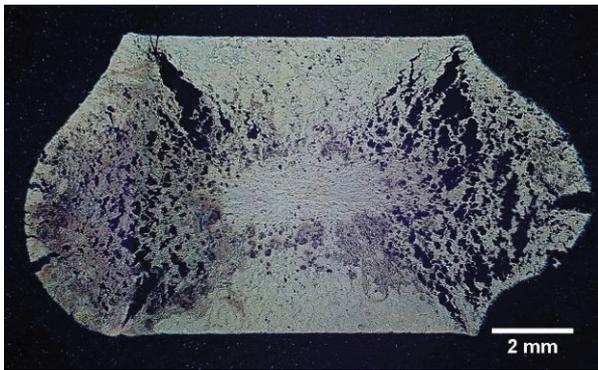
**Figure 3** The sample of the Ni-22Al-0.5B alloy in cast state after compression test
