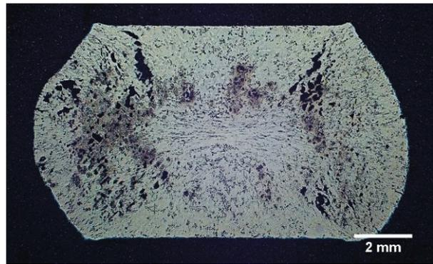
**Figure 4** The sample of the Ni-24Al-0.5B alloy in cast state after compression test
