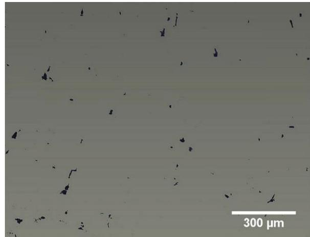
**Figure 2** A detail of the directionally solidified structure of the Ni-24Al-0.5B alloy
