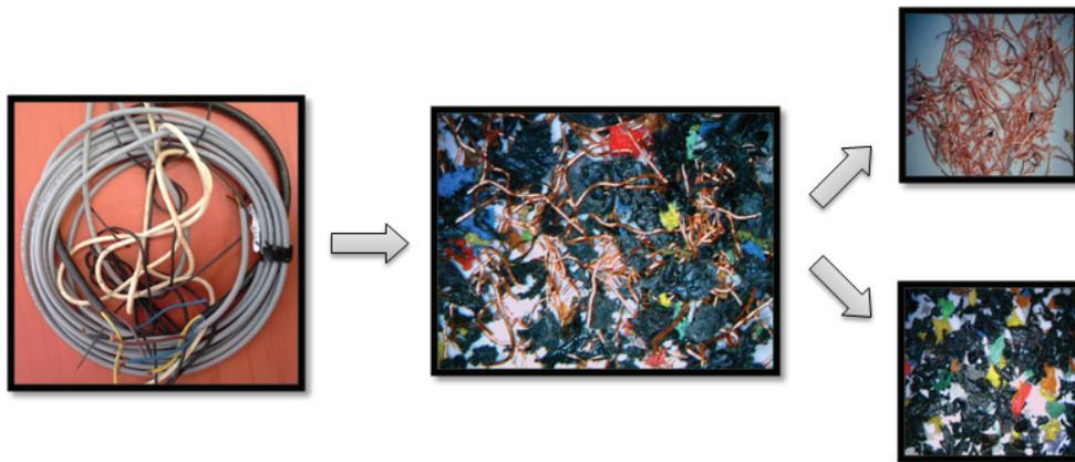
**Figure 1** Schematic representation of electrical waste grit formation and its separated components
