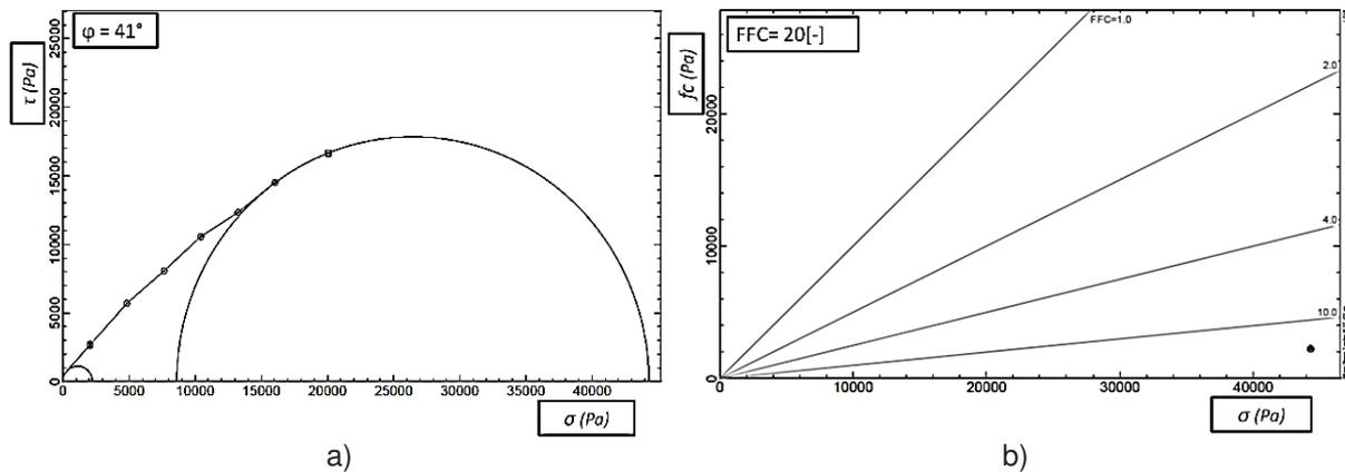
**Figure 2** Results a) angle of internal friction  $\varphi$  , b) flowability FFC
