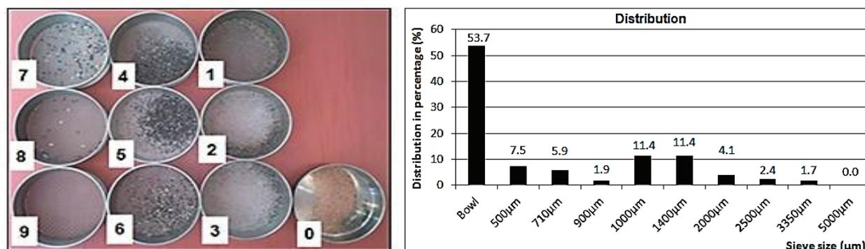
**Figure 4** Representation of the sieve sorting result
