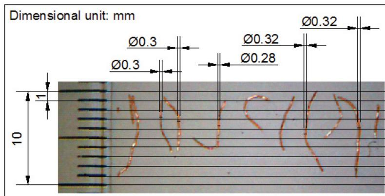
**Figure 3** Dimensional detail of fine copper wires on a scale of 2.5:1
