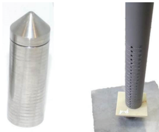
Figure 4 Impact test: impact hammer and test stand
