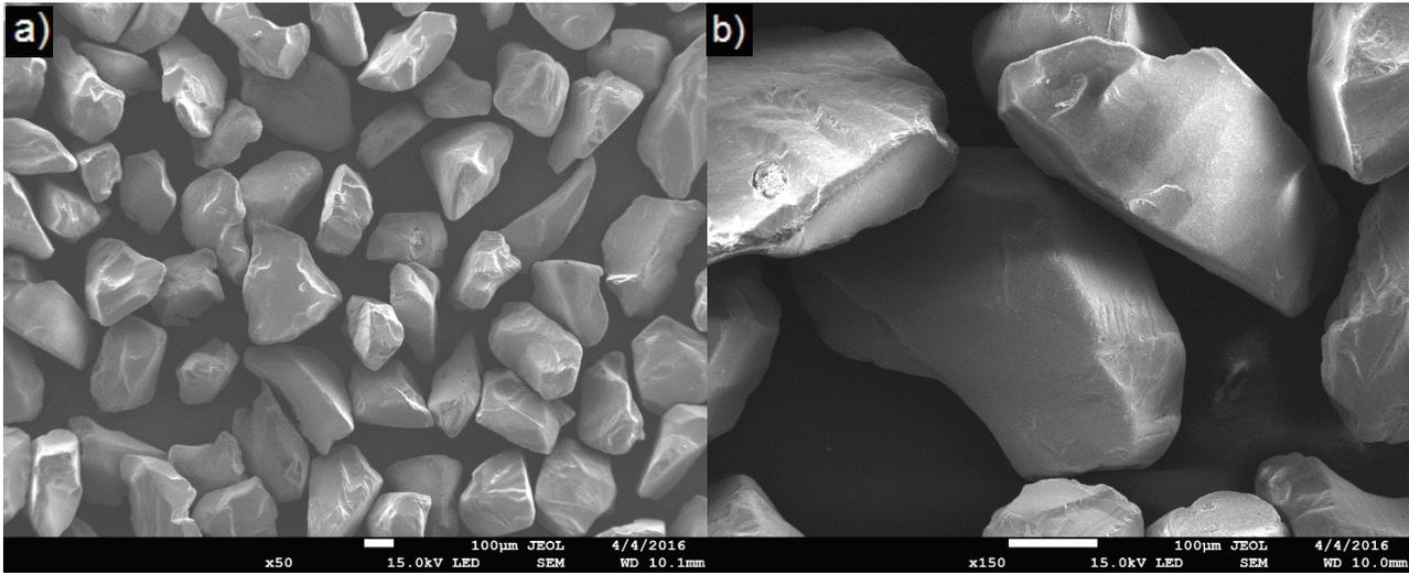
**Figure 2** SEM images of the abrasive grains (garnet # 80 E)
