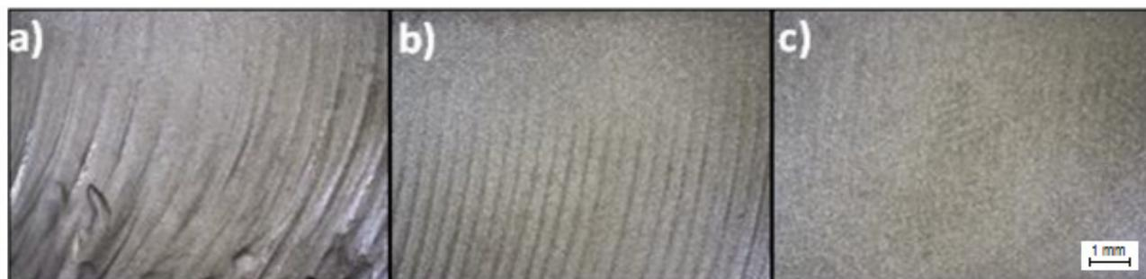
**Figure 1** Surface structure of C45 steel produced by abrasive water jet cutting assessed as:
