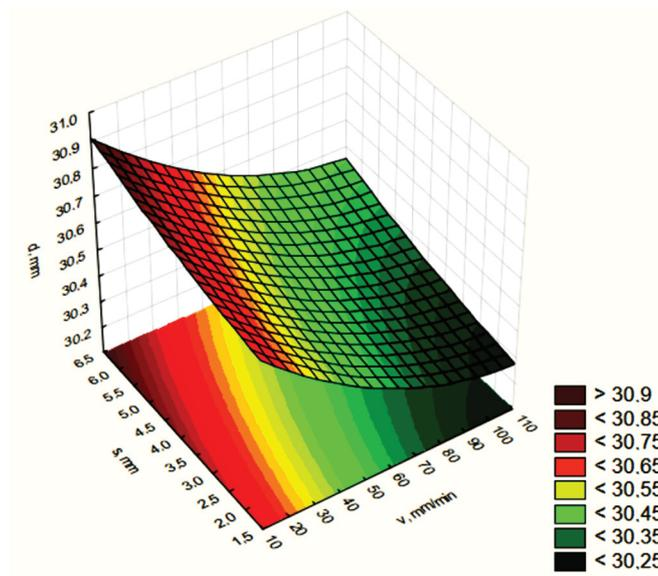
**Figure 4** Relationship between the hole diameter, the cutting speed and the distance between the nozzle and the workpiece at  $m_a = 340$  g/min
