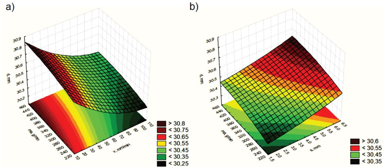
**Figure 3** a) Relationship between the hole diameter, the cutting speed and the abrasive mass flow rate at  $s = 4$  mm, b) Hole diameter vs. the distance between the nozzle and the workpiece vs. the abrasive mass flow rate at  $v = 60$  mm/min
