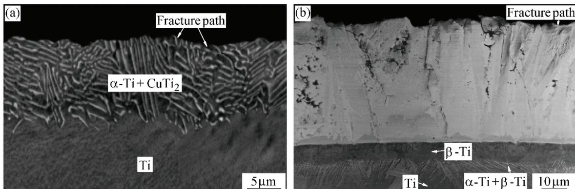
**Figure 5** Cross-section of the fracture surface from titanium side of the joints processed at 875 °C for 60 min cooled with two different cooling rates: (a) 3 and (b) 60 °C·min<sup>-1</sup>
