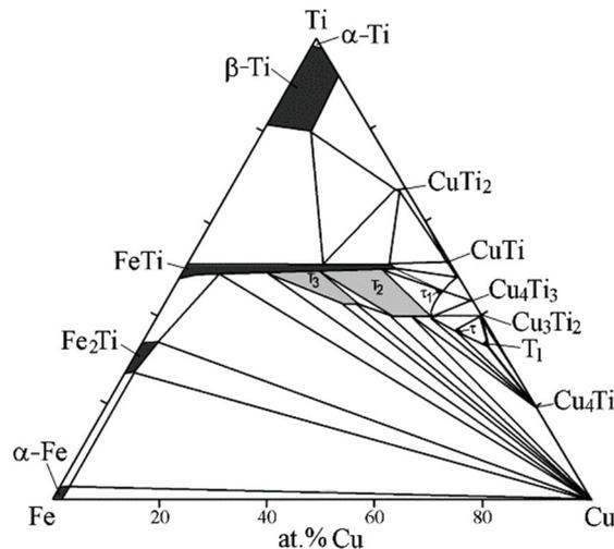
**Figure 1** Isothermal cross-section through the ternary phase diagram Cu-Ti-Fe at 850 °C [13]
