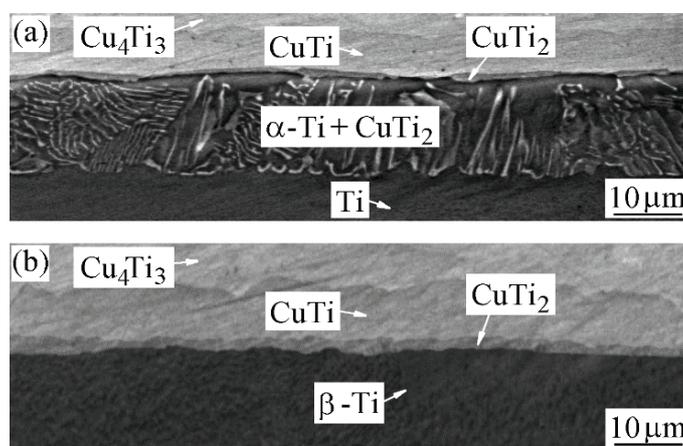
**Figure 3** Microstructure of the layers adjacent to titanium cooled at rates: (a) 3 and (b) 60 °C·min<sup>-1</sup>
