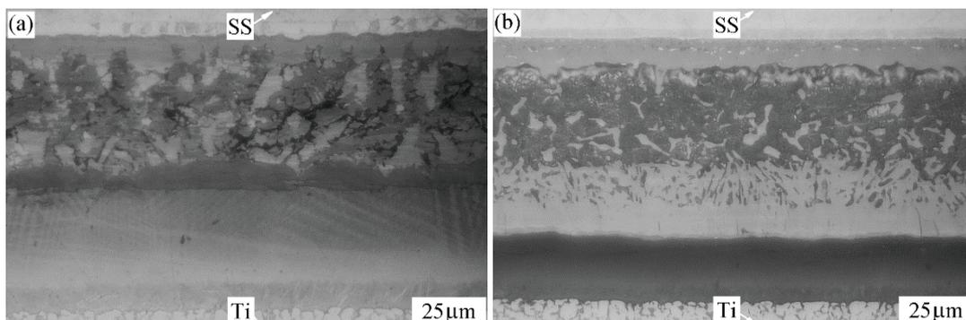
**Figure 2** Optical micrographs of the joints prepared at (a) 875 °C and (b) 900 °C for 60 min
