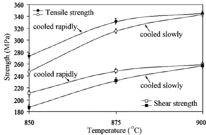
**Figure 4** Relation between average tensile and shear strengths of the joints processed for 60 min, type of cooling, and bonding temperature
