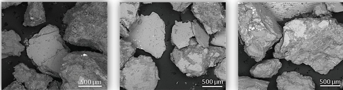
**Figure 1** SEM a photograph of AGV sample. (Left - feed, middle - concentrate, right - waste)
