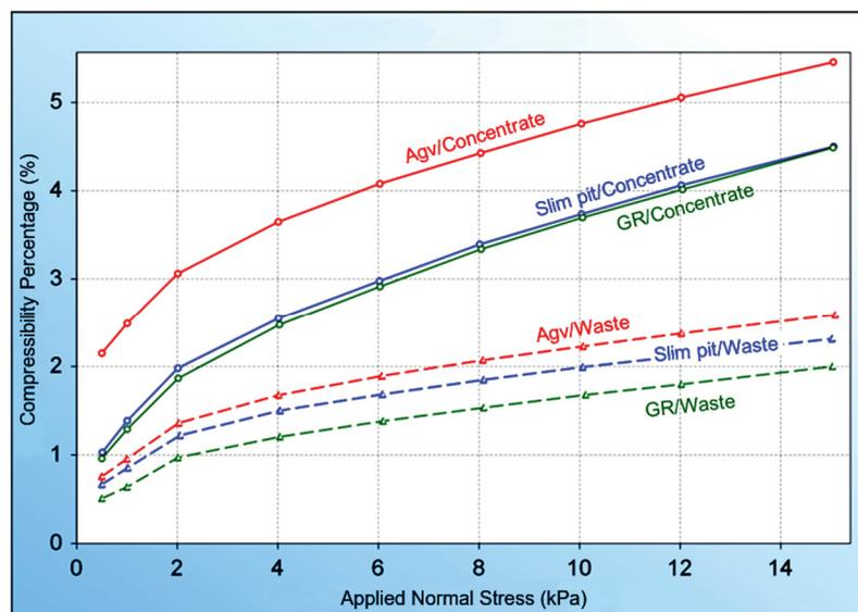
**Figure 2** Compressibility tests for samples after magnetic separation
