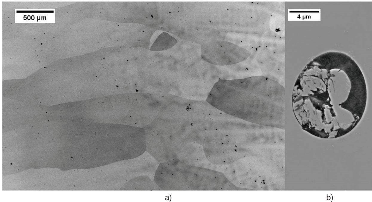
**Figure 1** Microstructure (EDX analysis) of the as-cast sample: a) overview and b) detail of a pore
