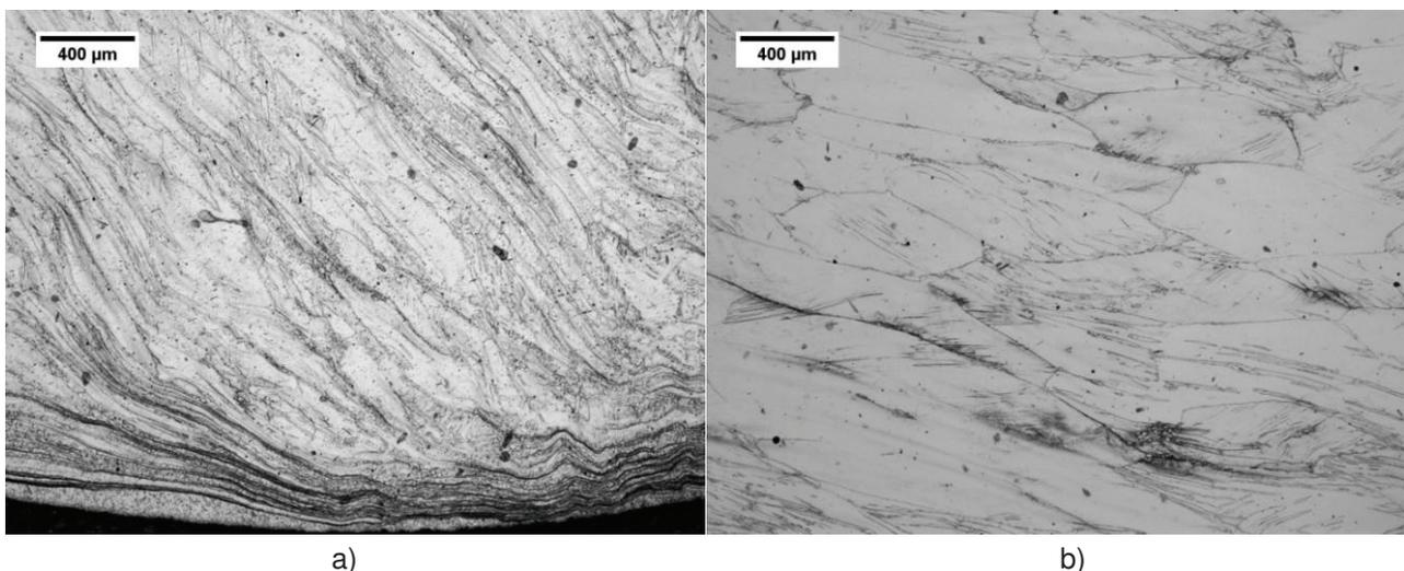
**Figure 2** Microstructure of the forged piece: a) on the edge and b) in the central part
