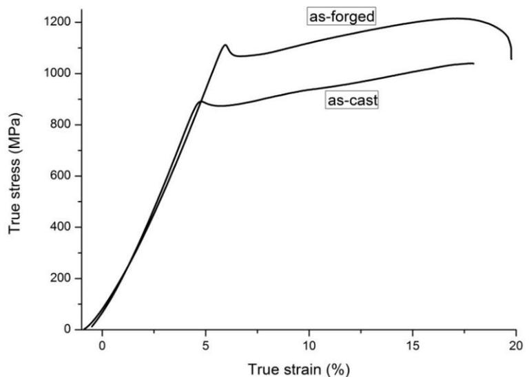
**Figure 3** True stress - true strain curves for as-cast and as-forged material
