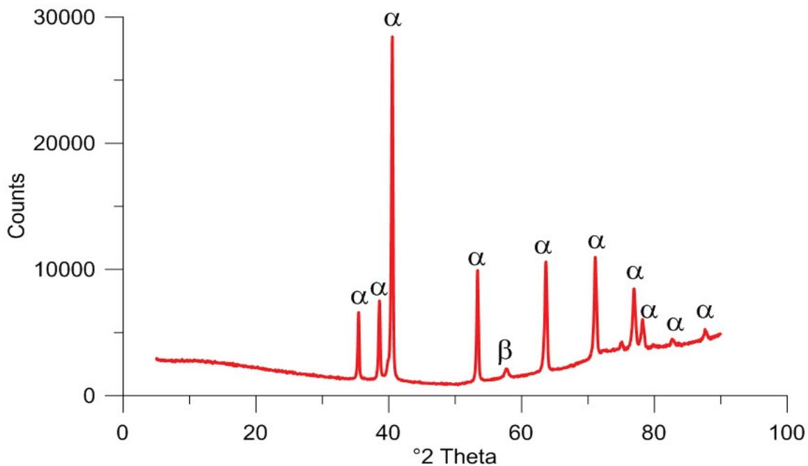
**Figure 3** XRD pattern of Ti-6Al-4V alloy prepared by SLM and subsequent heat treatment
