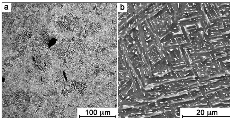
**Figure 2** Microstructures of SLM Ti-6Al-4V
