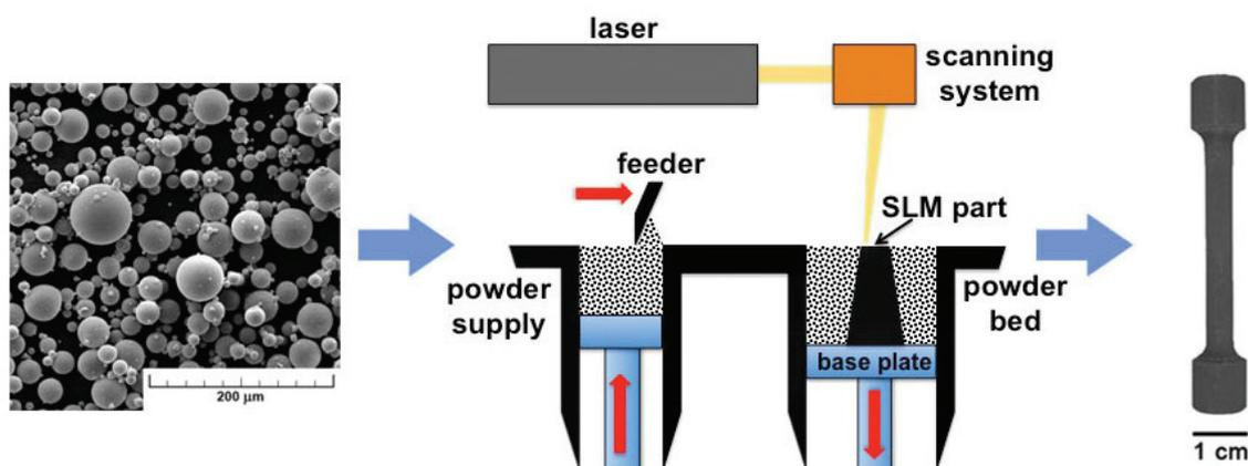
**Figure 1** SLM process schema with an input powder material and an output tensile specimen
