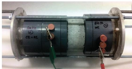
**Figure 2** Experimental design of EIS measurement
