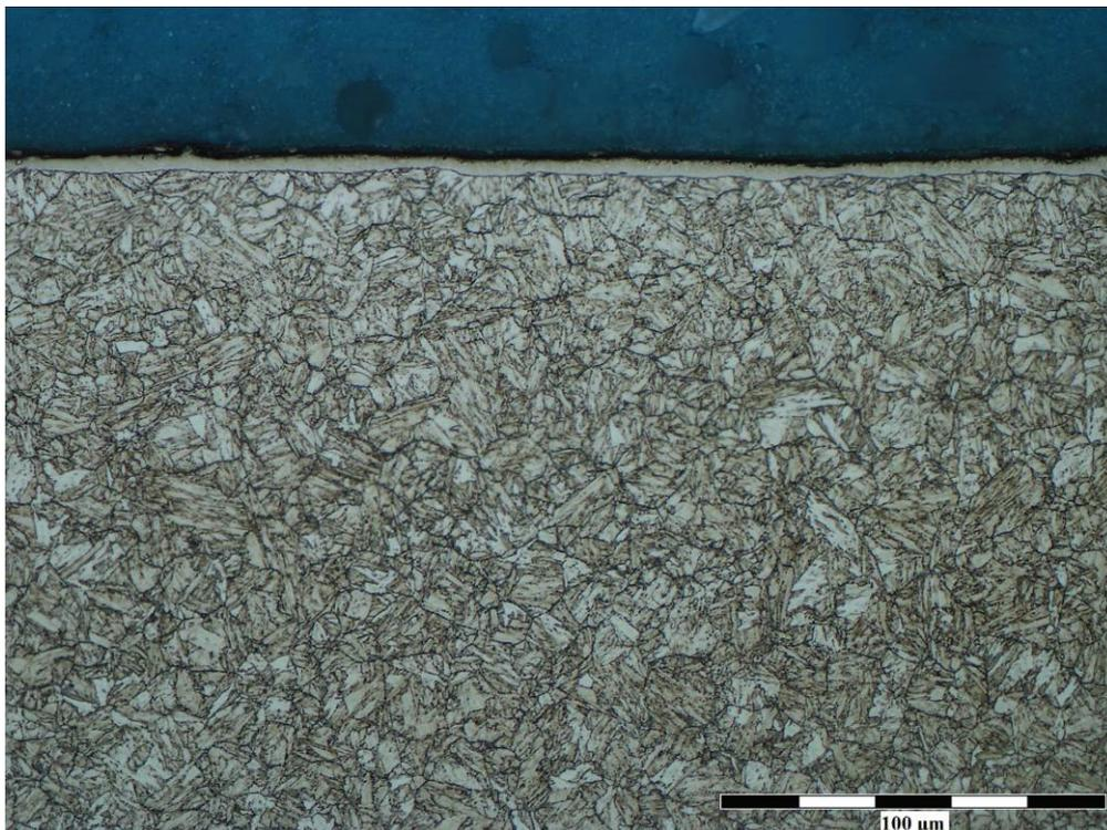
**Figure 3** Microstructure of plasma nitrided sample; PN 500 °C/30 h/280 Pa
