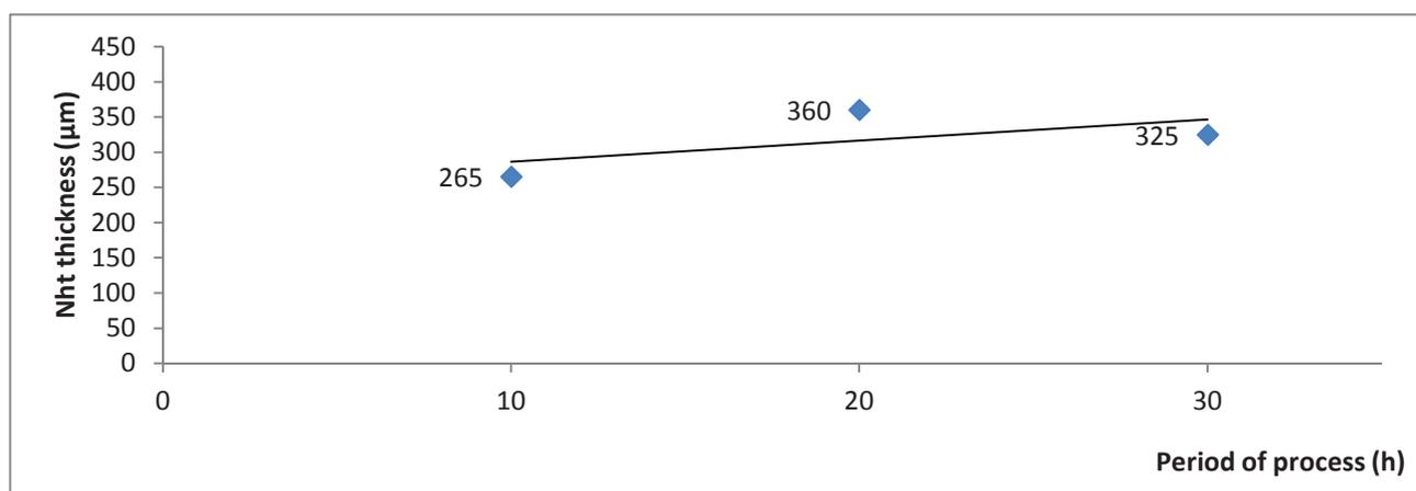
**Figure 5** The thickness of nitrided layers
