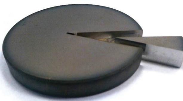
**Figure 1** Plasma nitrided DIN 16MnCr5 steel sample
