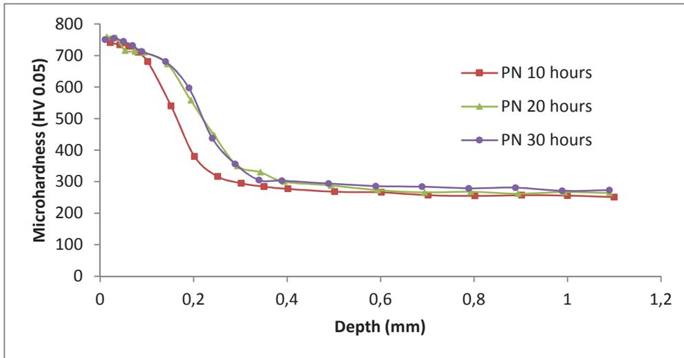
**Figure 4** The microhardness profiles of plasma nitrided DIN 16MnCr5 steel
