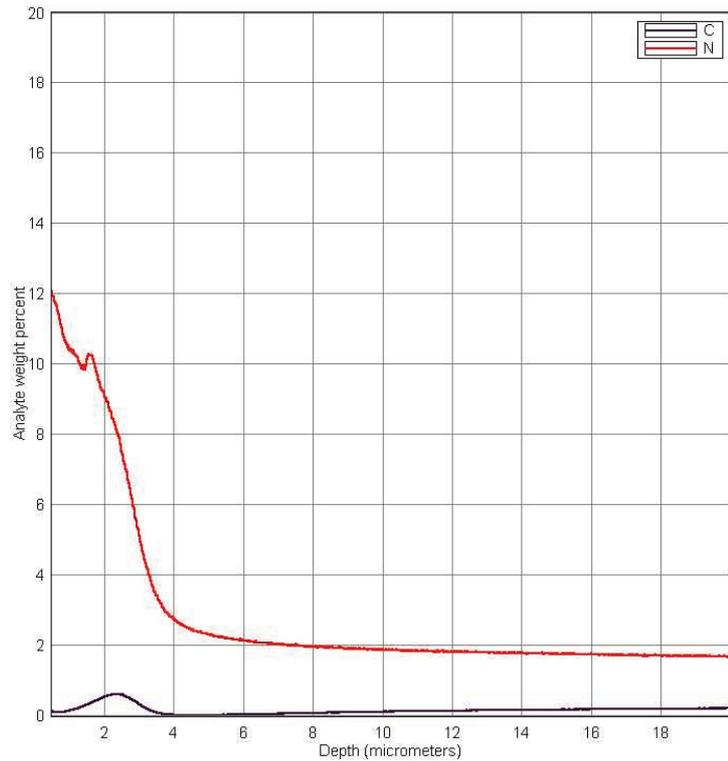
**Figure 2** The concentration profile plasma nitride DIN 16MnCr5 Steel (PN 5 h)
