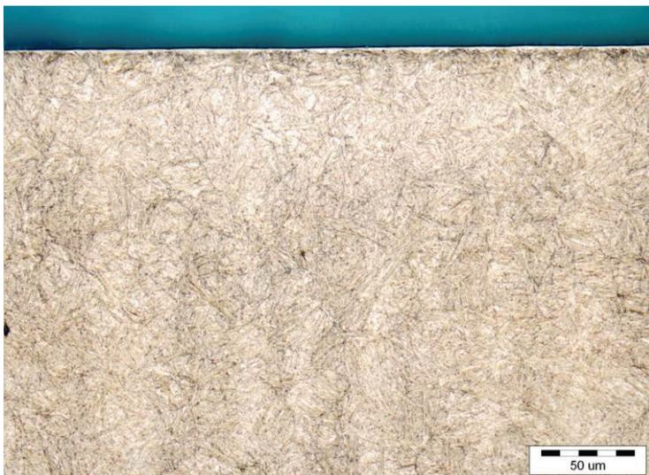
**Figure 1** NITAL etched cross-sectional structure of heat-treated sample after plasma nitriding process; 4 hours
