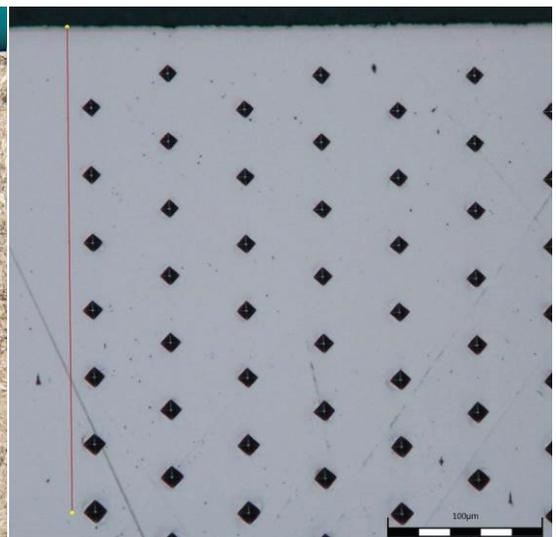
**Figure 2** Indentation pattern of microhardness measurement
