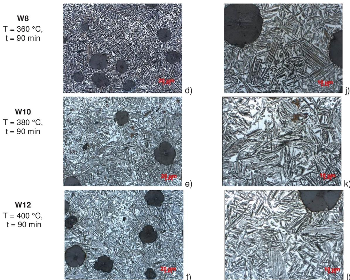
**Figure 3** Photos of microstructures of the examined cast iron after different variants of heat treatment, a-f) lower magnification, g-l) double magnification
