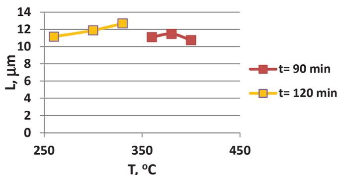
**Figure 5** Plotted changes in the length of ferrite needles as a function of the time and temperature of austempering
