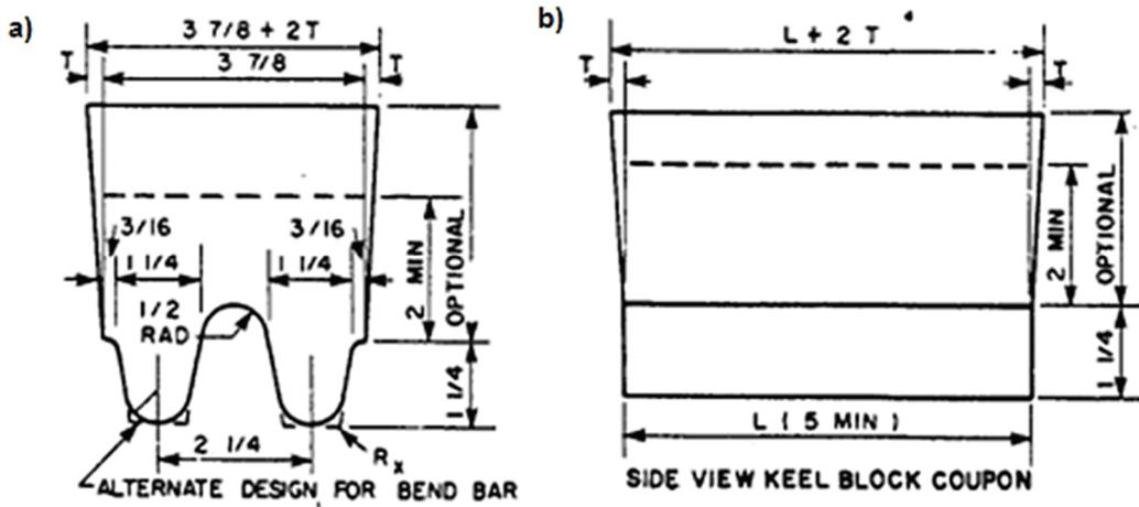
Figure 1 A schematic of the keel block cast acc. to ASTM A897, a) front view, b) side view
