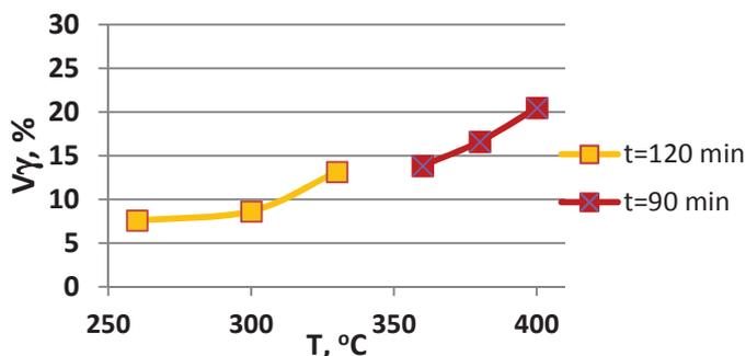
**Figure 4** Plotted changes in the relative volume fraction of austenite as a function of the temperature of austempering
