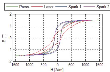
**Figure 8** Hysteresis curves for different processing at 1.5 T and 50 Hz
