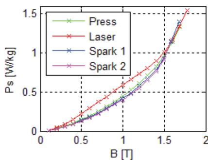
**Figure 14** Dependency of total magnetic losses  $P_s$  on magnetic flux density  $B$  at 15 Hz
