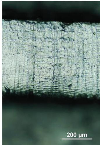
**Figure 6** OM detail of edge sheet after laser cutting
