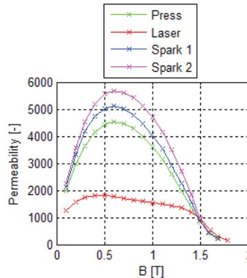
**Figure 12** Dependency of permeability on magnetic flux density at 15 Hz
