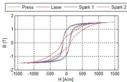
**Figure 8** Hysteresis curves for different processing at 1.5 T and 50 Hz
