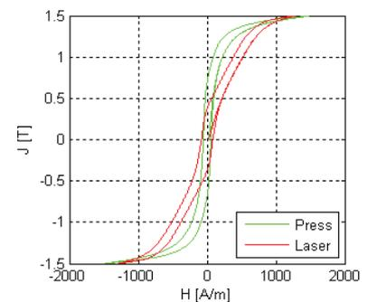
**Figure 16** Hysteresis curves measured at RemaGRAPH
