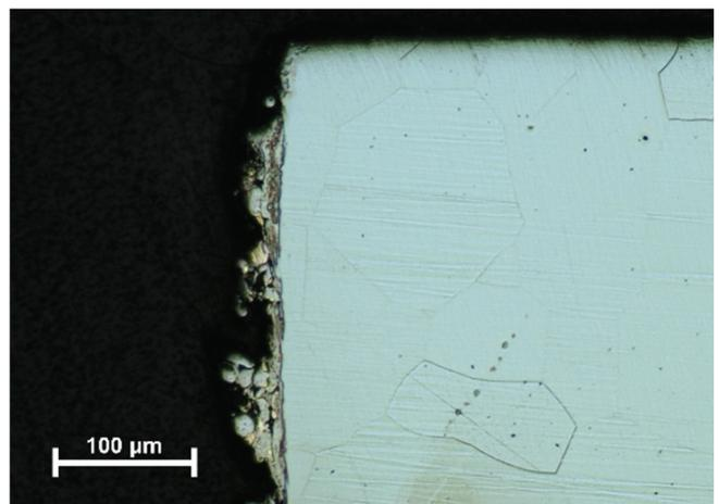
**Figure 4** OM sheet, spark cutting 2, etching
