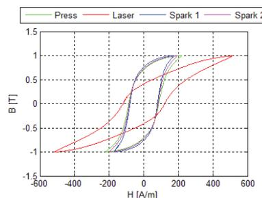
**Figure 9** Hysteresis curves for different processing at 1.0 T and 50 Hz
