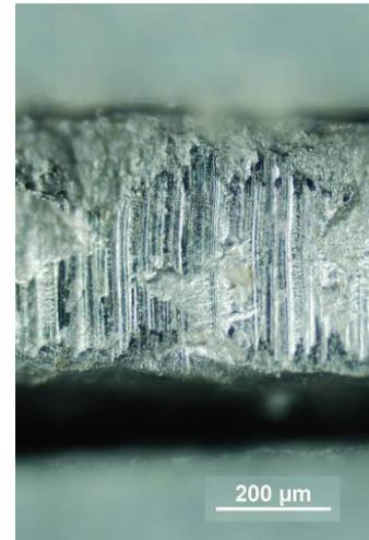
**Figure 7** OM detail of edge sheet after punching
