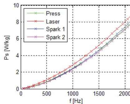
**Figure 15** Comparison total magnetic losses  $P_s$  on frequencies
