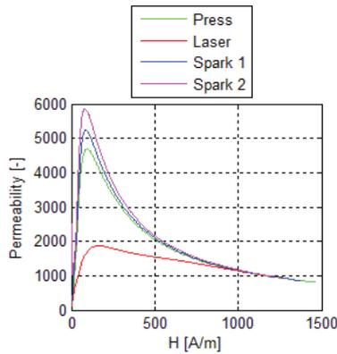
**Figure 11** Dependency of permeability on magnetic field strength  $H$  measured at RemaGRAPH
