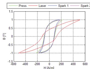
**Figure 9** Hysteresis curves for different processing at 1.0 T and 50 Hz
