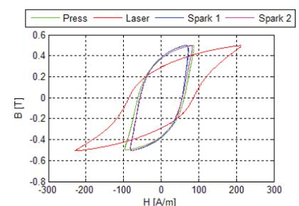
**Figure 10** Hysteresis curves for different processing at 0.5 T and 50 Hz
