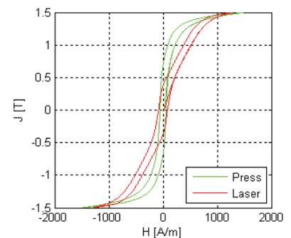
**Figure 16** Hysteresis curves measured at RemaGRAPH
