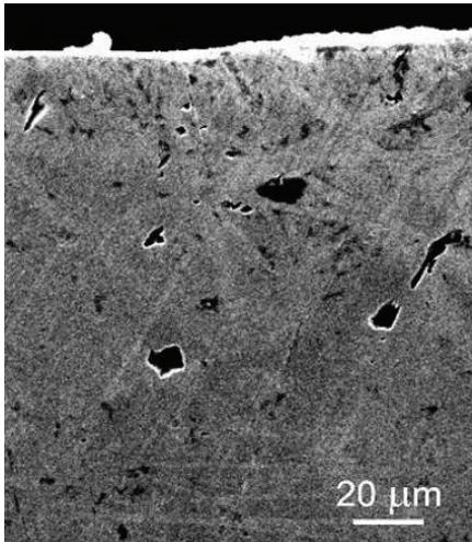
**Figure 5** SEM sheet after laser cutting (upper edge influenced)
