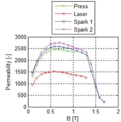
**Figure 13** Dependency of permeability on magnetic flux density at 400 Hz
