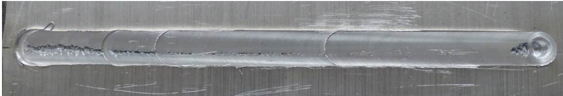
Figure 3 An example of friction stir welded joint with incorrect parameters - visible welding defects
