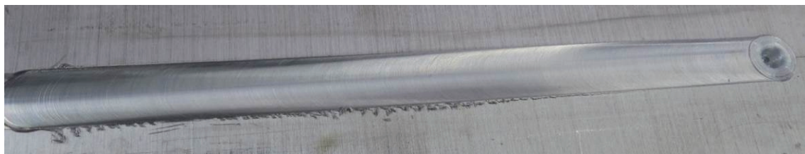
Figure 4 An example of friction stir welded joint with correct parameters - lack of welding defects
