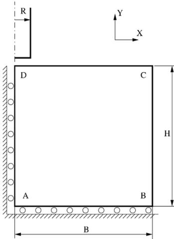
**Figure 3** Scheme of axisymmetric FEM model
