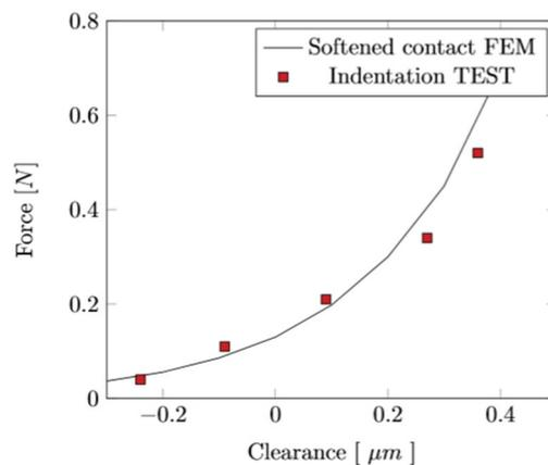
**Figure 4** Softened contact FEM, Indentation test
