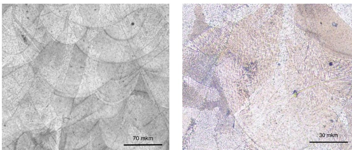
**Figure 2** Microstructure of cross-section specimen after SLM
