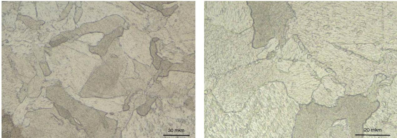
**Figure 3** Microstructure of specimen after SLM and heat treatment
