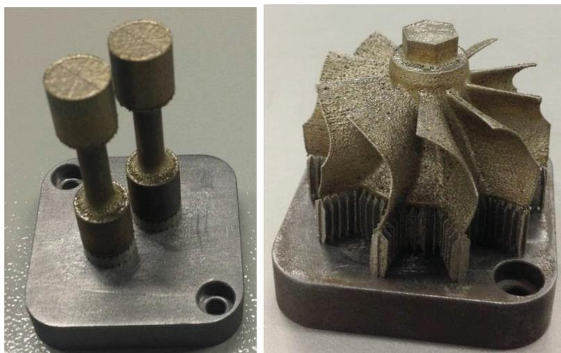
**Figure 4** Images of specimens for tensile tests and turbine wheel manufactured by selective laser melting of 316L stainless steel
