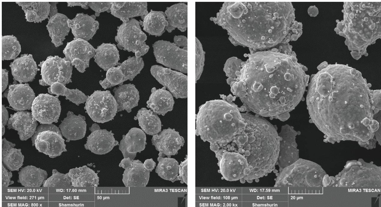
**Figure 1** SEM-images of steel 316L powder particles
