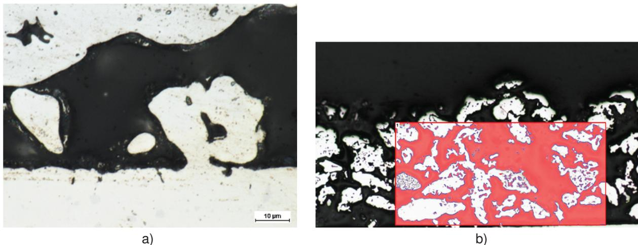
**Figure 1** a) The microstructures of the sample porous structure. Not etched;
