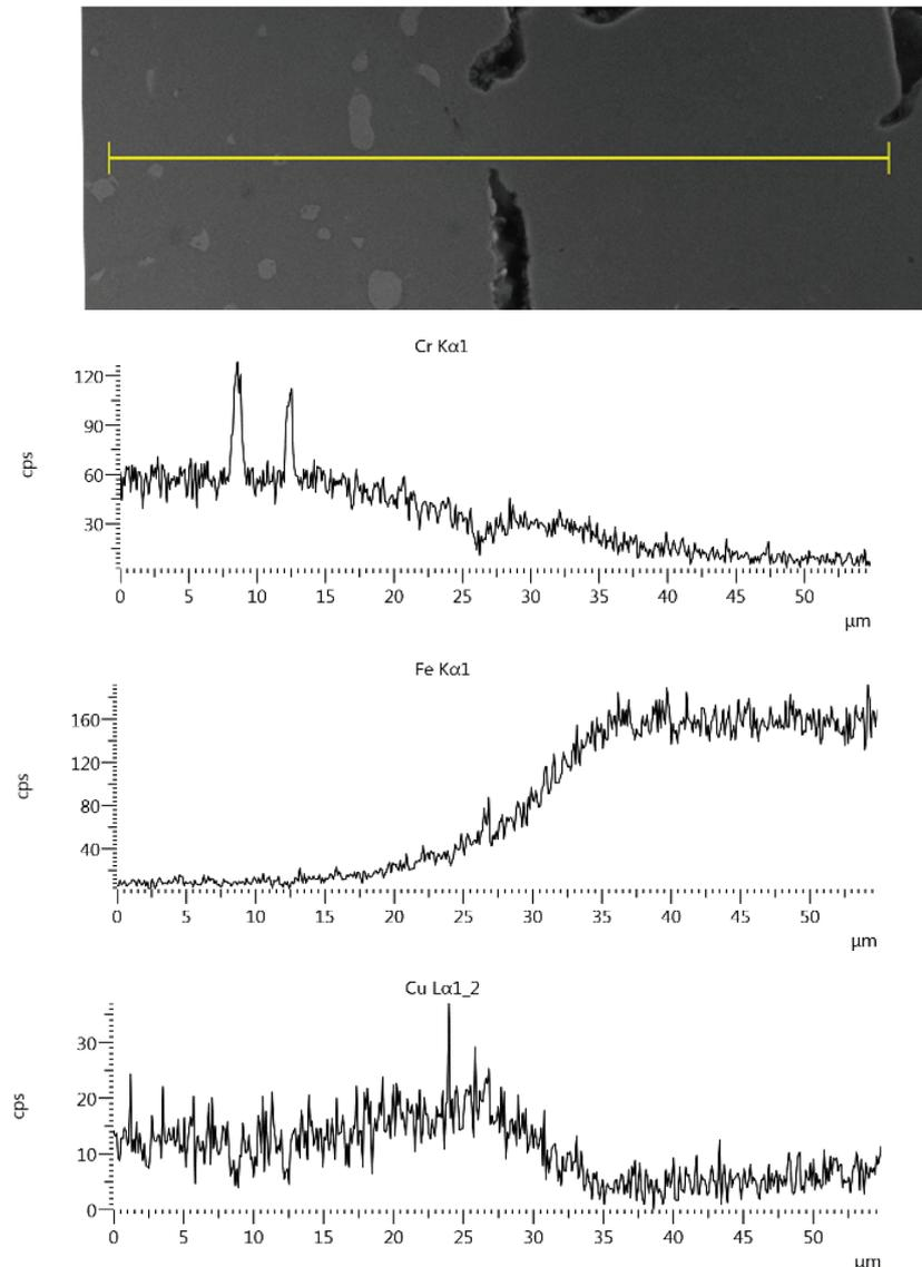
**Figure 2** SEM examination of the diffusion bridge between HASTELLOY<sup>®</sup> and Distaloy SE grain
