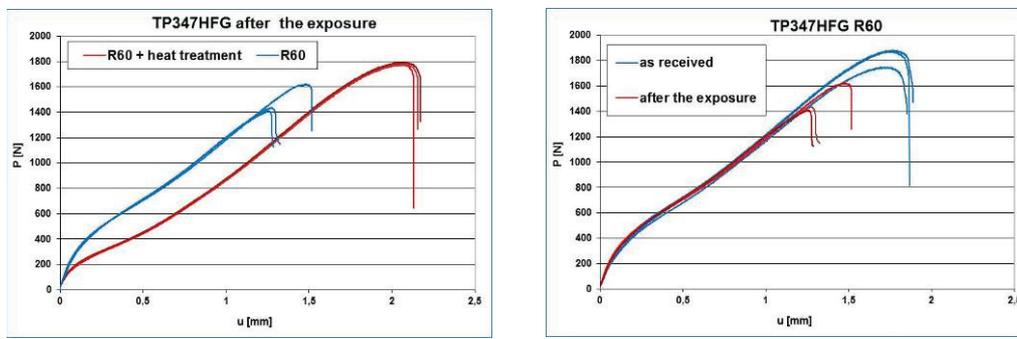
**Figure 7** Force versus displacement of bend tube TP347HFG in state as received and after the exposure
