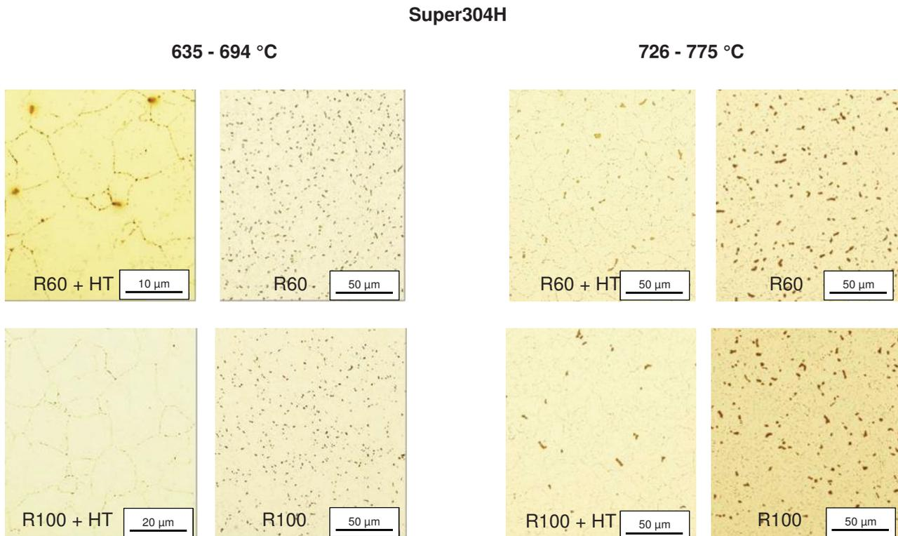
**Figure 6** Comparison of the structure specimen Super 304H as received after exposure in two location of boiler
