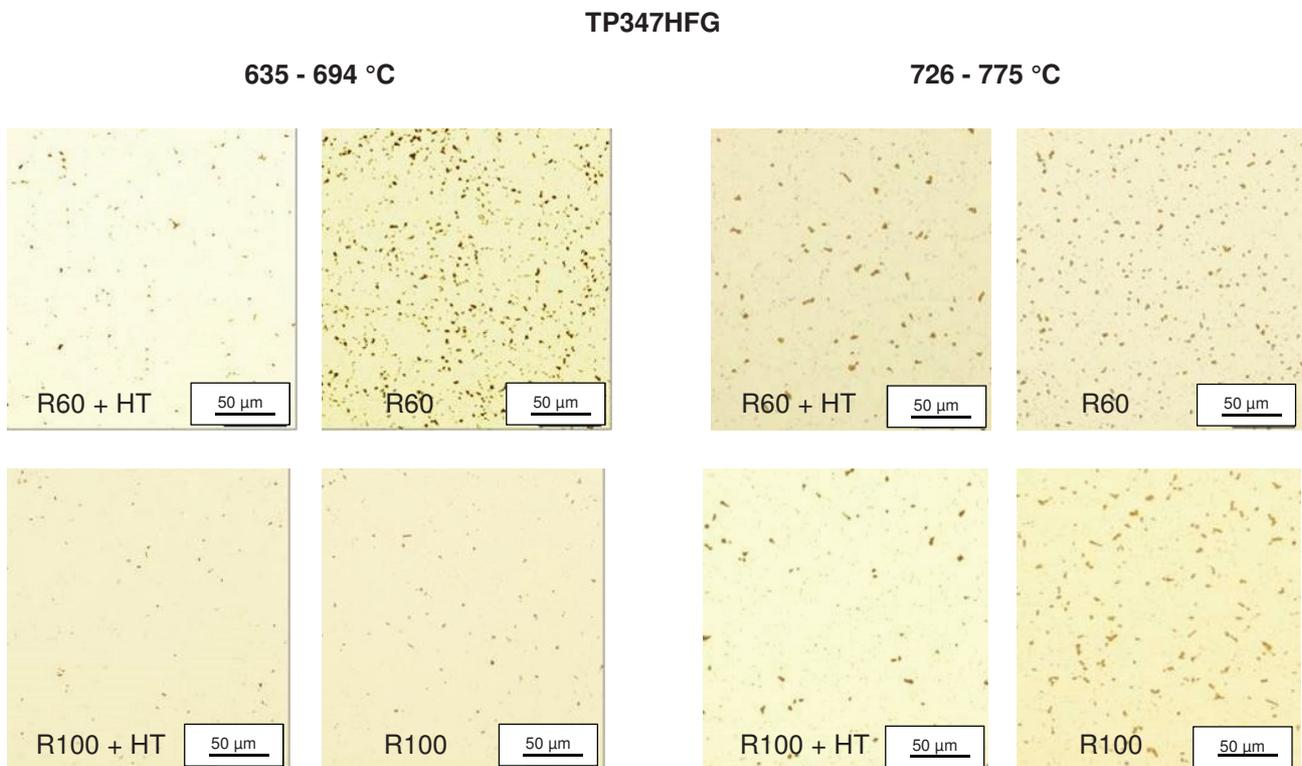
**Figure 4** Comparison of the structure specimen TP347HFG as received after exposure in two location of boiler
