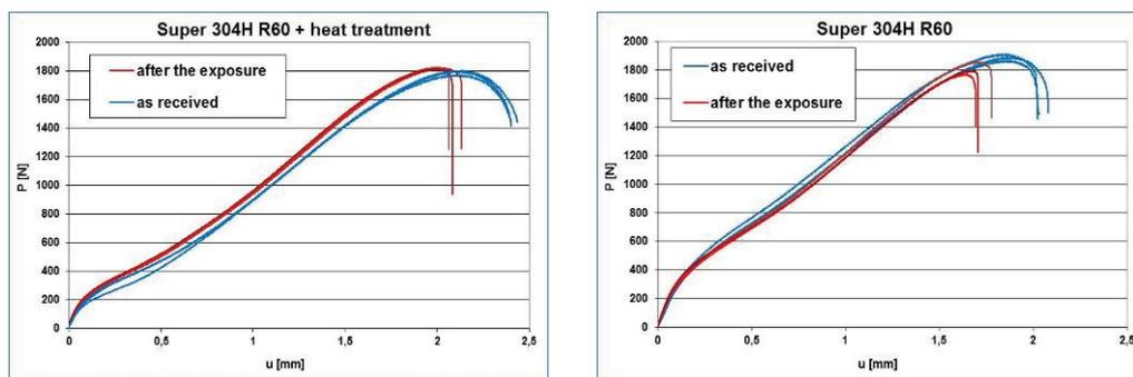
**Figure 9** Force versus displacement of bend tube Super 304H in state as received and after exposure
