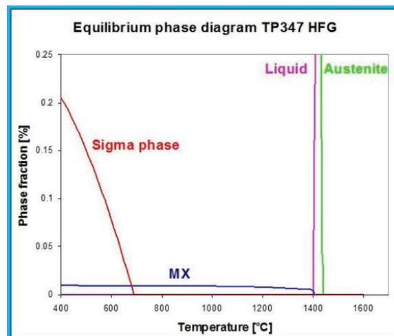
**Figure 1** Equilibrium phase diagram TP347 HFG calculated with MatCalc software [1]
