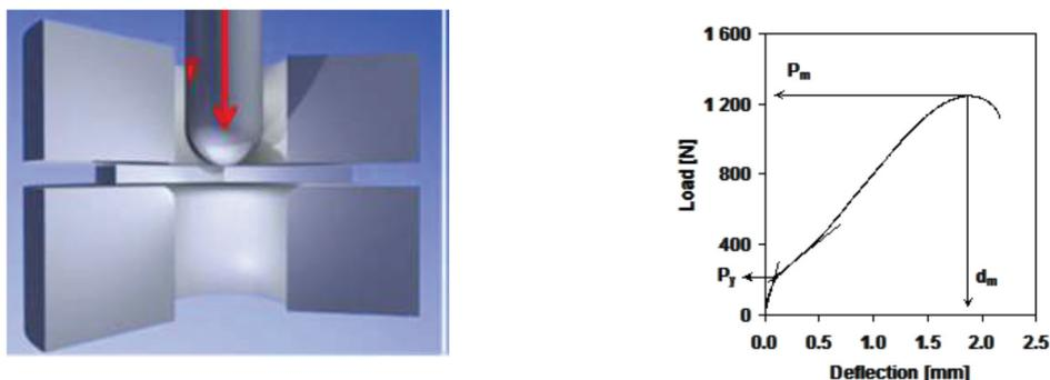
**Figure 3** Principle of small punch test and typical SPT record
