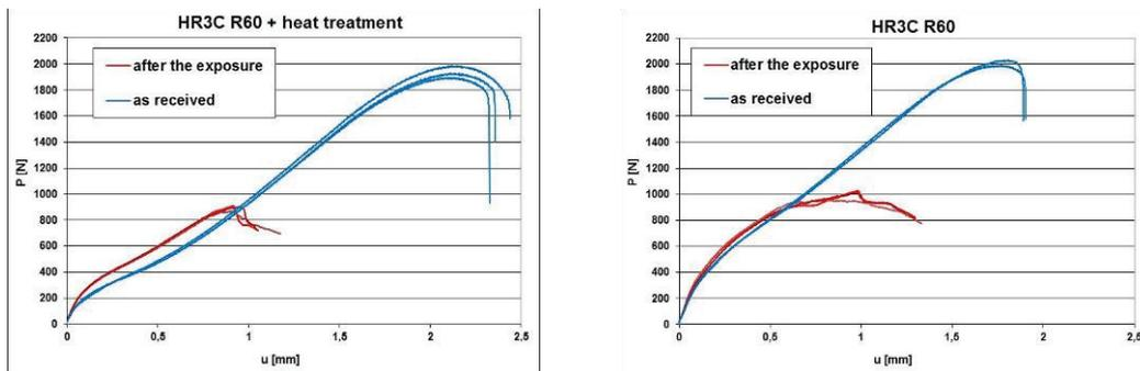
**Figure 8** Force versus displacement of bend tube HR3C in state as received and after exposure
