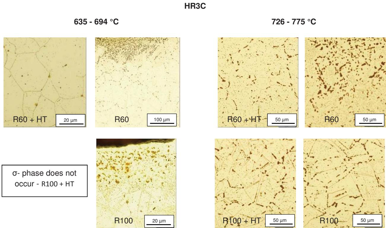
**Figure 5** Comparison of the structure specimen HR3C as received after exposure in two location of boiler
