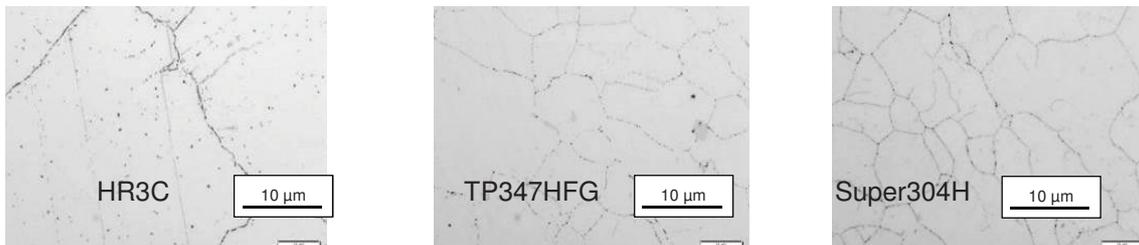
**Figure 10** The structure without  $\sigma$ -phase in the straight part on bend tubes after the exposure
