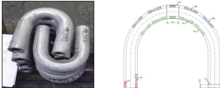
**Figure 2** Samples under study and cutting plan
