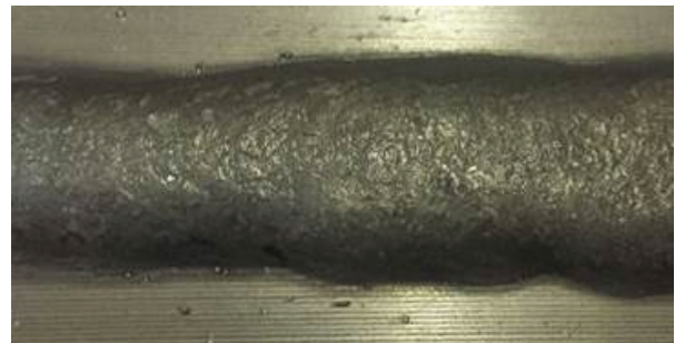
Figure 4 Image of the exterior surface of the welding E_l = 20.7 kJ/cm
