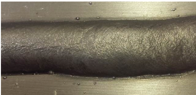
Figure 3 Exterior surface of the welding E_l = 15 kJ/cm
