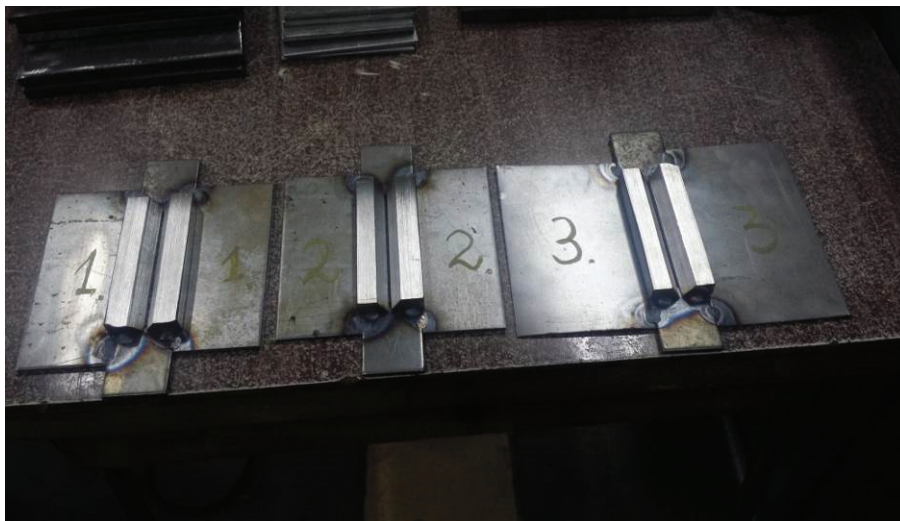
Figure 1 Position of the components to be welded
