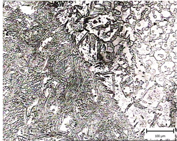
Figure 6 Microstructure of the weld-heat affected zone interface for E_l = 15 kJ / cm
