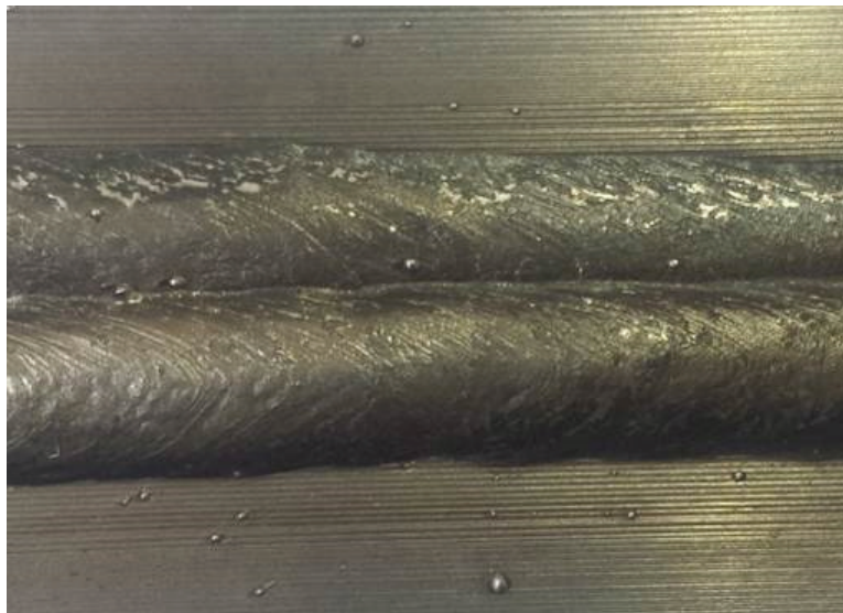
Figure 2 The aspect of the exterior surface of the welded joint E_l = 10 \text{ kJ / cm}
