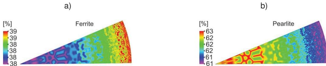
**Figure 4** The percentage fraction of ferrite (a) and pearlite (b) of the 30MnB4 steel bar cross-section
