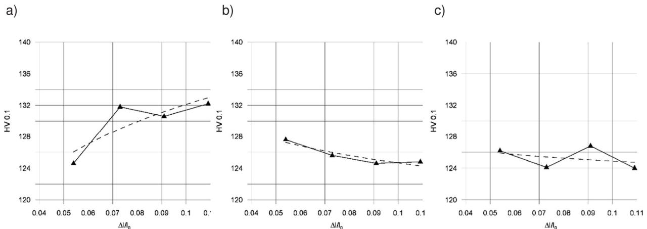
**Figure 5** The microhardness distributions in different zones of longitudinal sections of hydromechanically bulged axisymmetric components made from copper tubes at relative ratios  $\Delta l/l_0=0.054$ ;  $\Delta l/l_0=0.073$ ;  $\Delta l/l_0=0.091$  and  $\Delta l/l_0=0.109$ : a) zone I, b) zone II, c) zone III
