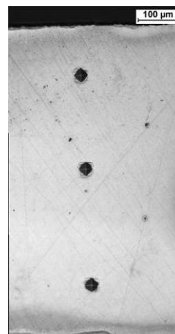
**Figure 4** Indentations for microhardness measurements in zone III of longitudinal sections of hydromechanically bulged axisymmetric components made from copper tubes at relative ratios  $s_0/D=0.045$  and  $\Delta l/l_0 = 0.109$
