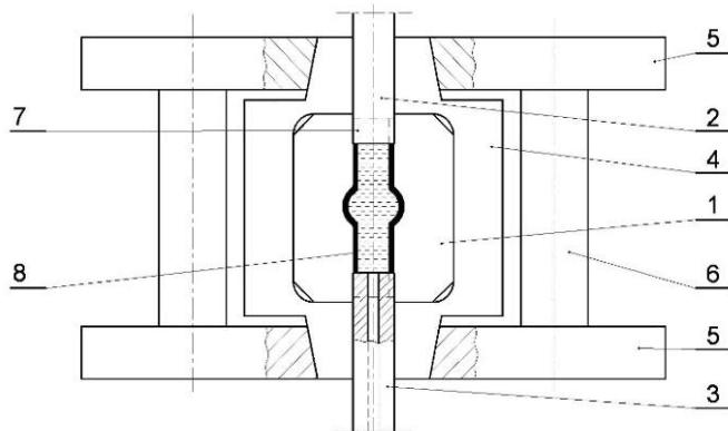
**Figure 1** Diagram of the main part of the hydromechanical bulge forming tool, where: 1- die insert, 2- upper punch, 3- lower punch, 4- half-die, 5- pressure platens, 6- guide-posts, 7- tube segment, 8- hydromechanically bulged axisymmetric component
