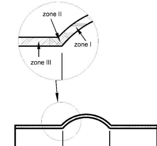
**Figure 3** Spacing of measurement zones for microhardness measurements in longitudinal sections of hydromechanically bulged axisymmetric components made from copper tubes at relative ratio  $s_0/D=0.045$
