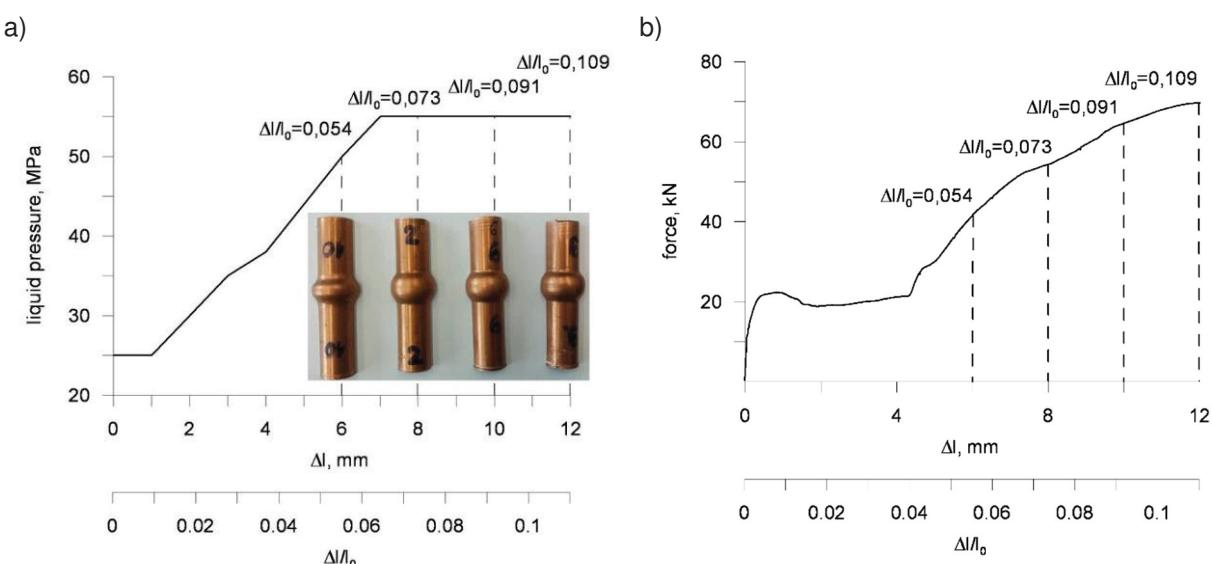
**Figure 2** Liquid pressure vs. displacement (a) and force vs. displacement obtained for hydromechanically bulged axisymmetric components at different ratios  $\Delta l/l_0$  ( $\Delta l/l_0=0.054$ ;  $\Delta l/l_0=0.073$ ;  $\Delta l/l_0=0.091$  and  $\Delta l/l_0=0.109$ )
