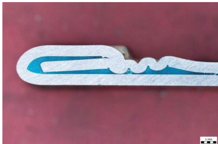
Figure 7 The hemmed joint with mechanical lock by grooving
