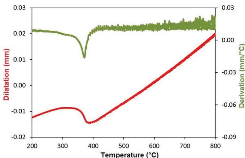
**Figure 2** Dilatation at cooling of the sample from the steel 25CrMo(S)4 at the cooling rate of 50 °C/s and the first derivation of the relevant curve in dependence on the temperature
