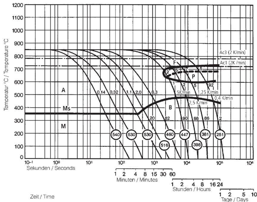
**Figure 8** CCT diagram of the steel Böhler V145 [12]
