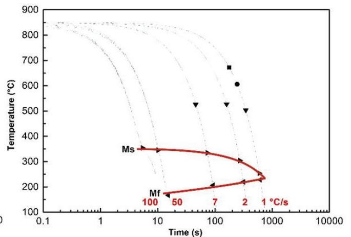
**Figure 4** Curves Ms and Mf determined by dilatometer for the steel 34CrMo(S)4
