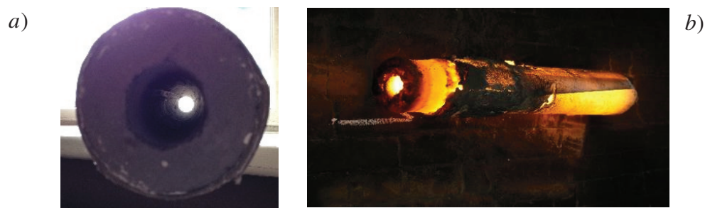
Figure 1 Nozzles: a) before the casting process, a) after the casting process
