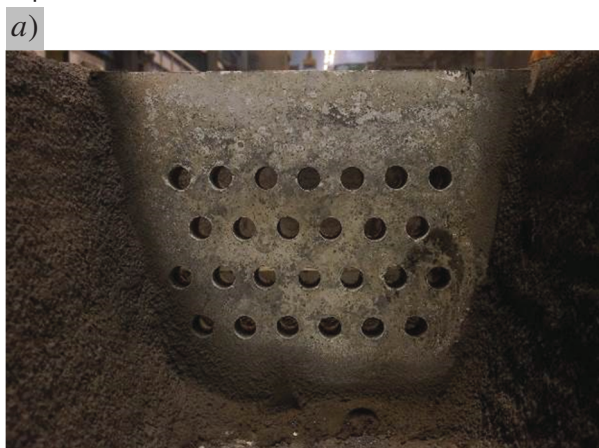
Figure 5 The tundish of the ceramic filter: a) before the filtration, b) after filtration
