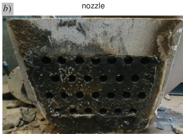
Figure 5 The tundish of the ceramic filter: a) before the filtration, b) after filtration
