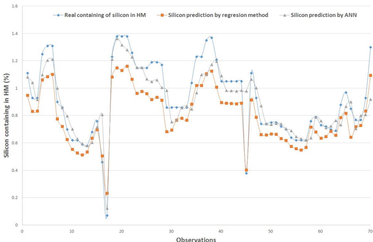
**Figure 1** Comparison of silicon prediction by different models with real measurement
