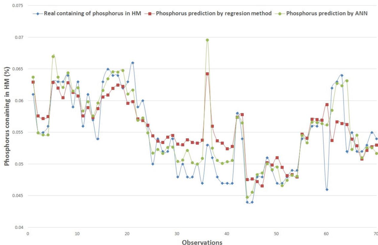
**Figure 3** Comparison of phosphorus prediction by different models with real measurement
