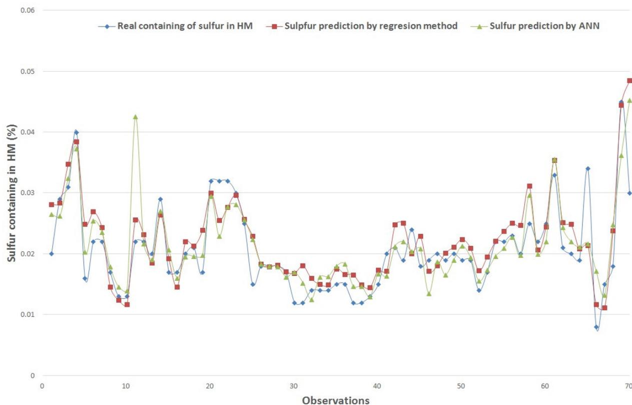
**Figure 2** Comparison of sulfur prediction by different models with real measurement
