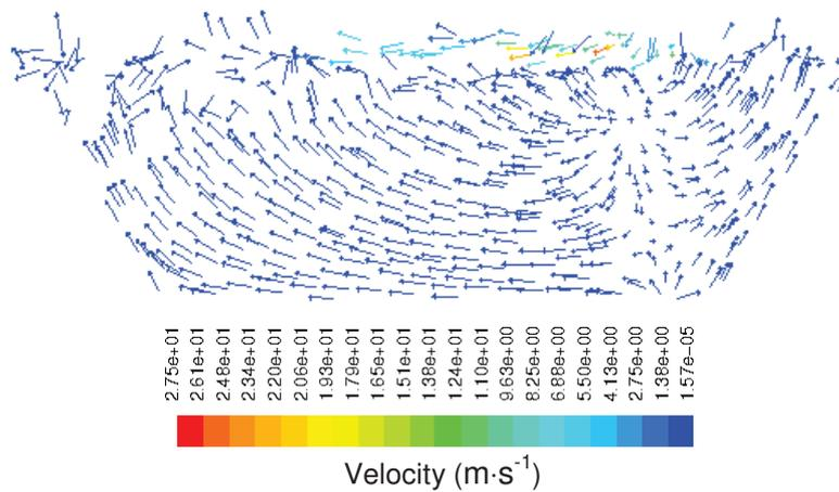
**Figure 3** Velocity field in the sectional view taken at a distance of 1.1 m to the right of the longitudinal central axis
