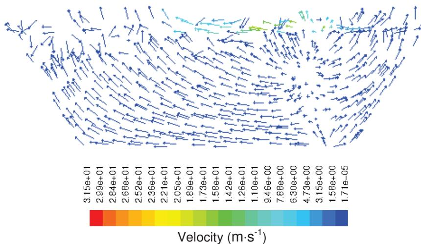
**Figure 4** Velocity field in the sectional view taken at a distance of 1.1 m to the left of the longitudinal central axis
