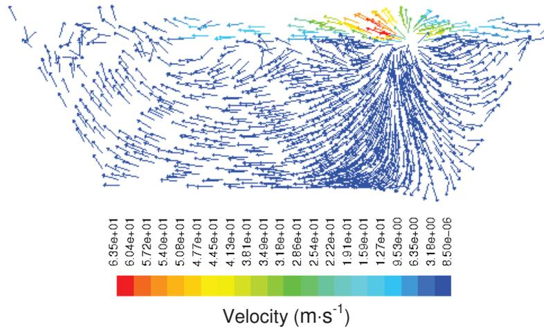
**Figure 2** Velocity field in cross section taken perpendicular to the surface of the melt in the longitudinal central axis of the hearth
