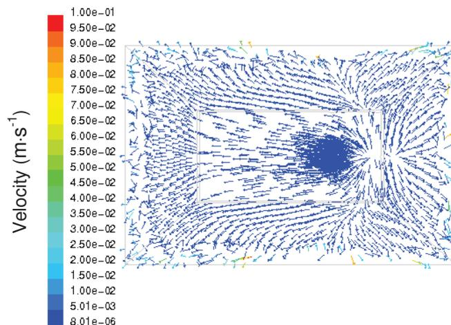
**Figure 6** Velocity field in the sectional view taken at a distance of 0.03 m from hearth surface
