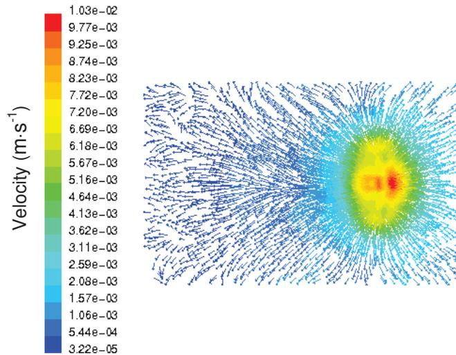
**Figure 5** Velocity field in the sectional view taken at a distance of 0.5 m under bath level
