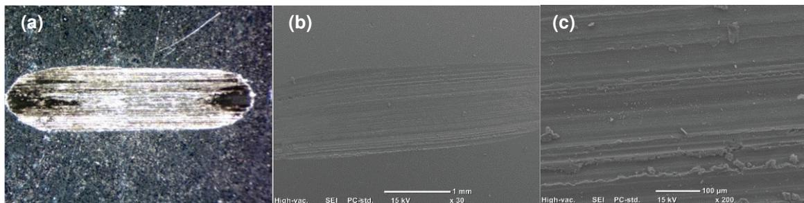
**Figure 7** (a) OM, (b) SEM and (c) SEM images of the worn surfaces taken from the 4 h of MA'd and sintered Al-7 wt.% Si-2 wt.% NbB-NbB<sub>2</sub>-Nb<sub>3</sub>B<sub>4</sub> composite
