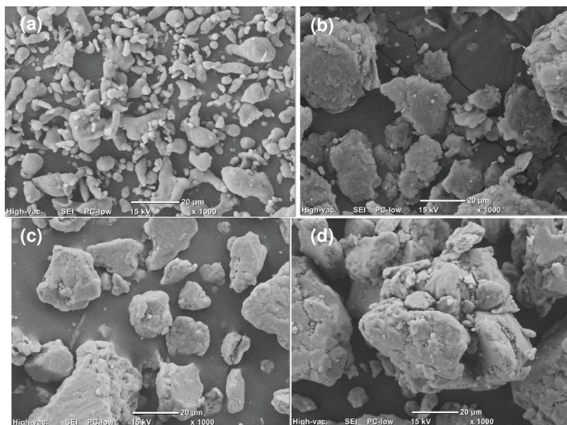
**Figure 2** SEM images of the as-blended and MA'd Al-7 wt.% Si-2 wt.% NbB-NbB<sub>2</sub>-Nb<sub>3</sub>B<sub>4</sub> powders: (a) as-blended, (b) MA'd for 1 h, (c) MA'd for 4 h and (d) MA'd for 8 h
