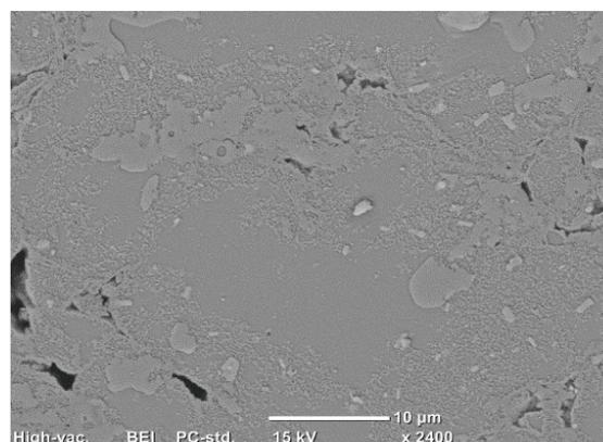
**Figure 6** SEM image of the 4 h of MA'd and sintered Al-7 wt.% Si-2 wt.% NbB-NbB<sub>2</sub>-Nb<sub>3</sub>B<sub>4</sub> composite
