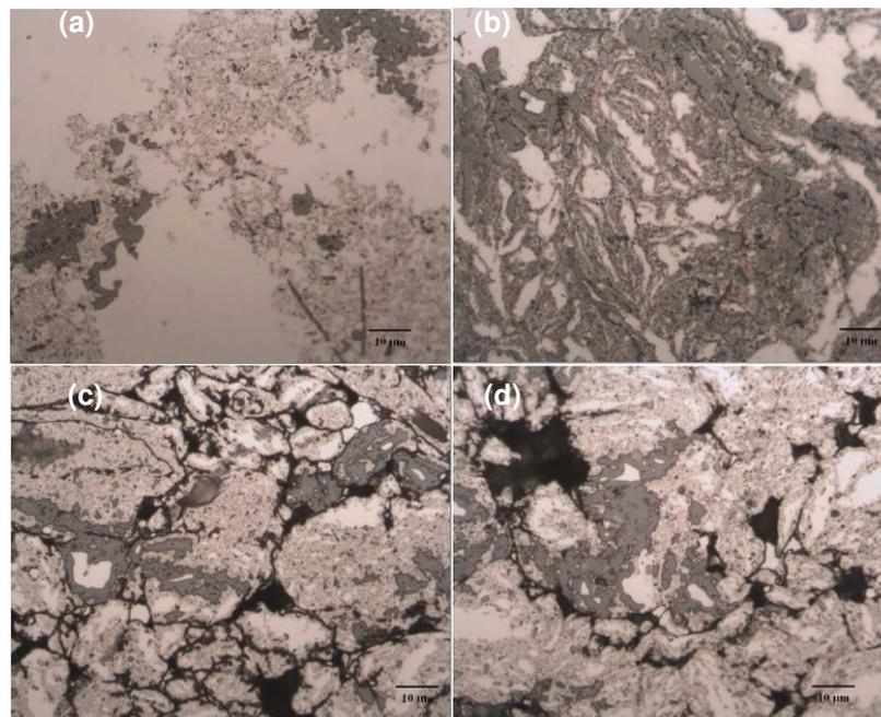
**Figure 5** OM images of the as-blended/MA'd and sintered Al-7 wt.% Si-2 wt.% NbB-NbB<sub>2</sub>-Nb<sub>3</sub>B<sub>4</sub> composites: (a) as-blended, (b) MA'd for 1 h, (c) MA'd for 4 h and (d) MA'd for 8 h
