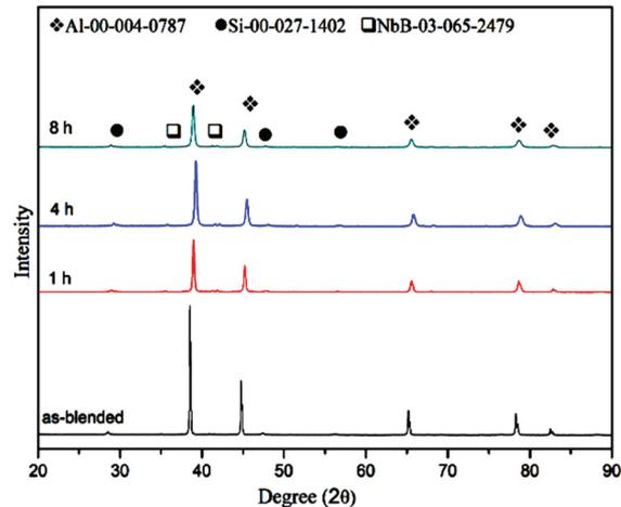
**Figure 1** XRD patterns of the as-blended and MA'd Al-7 wt.% Si-2 wt.% NbB-NbB<sub>2</sub>-Nb<sub>3</sub>B<sub>4</sub> powders at various durations (1, 4 and 8 h)
