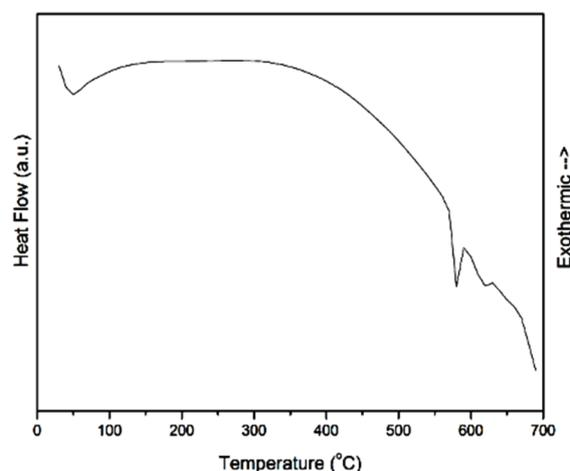
**Figure 4** DSC scan of the Al-7 wt.% Si-2 wt.% NbB-NbB<sub>2</sub>-Nb<sub>3</sub>B<sub>4</sub> powders MA'd for 4 h
