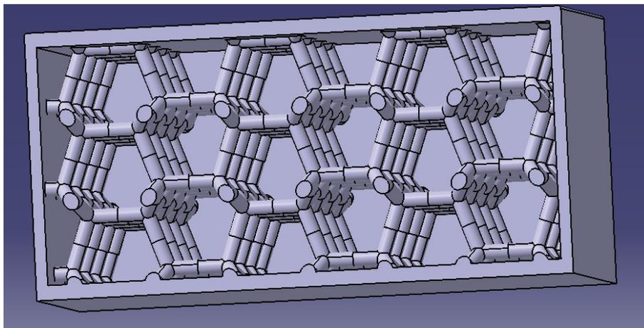
**Figure 3** Regular structure of diamond (case 1)
