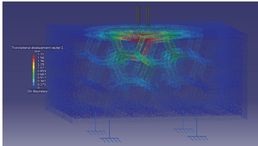
**Figure 5** Displacement of regular structure (case 1)
