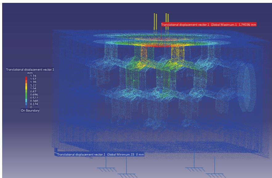
**Figure 8** Maximum displacement (case 2)
