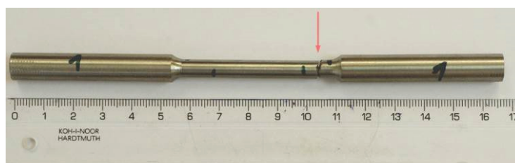
Figure 5 Tensile test sample after fracture
