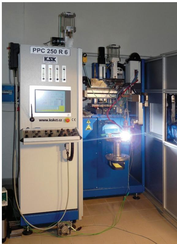
**Figure 1** Plasma hardfacing automate PPC 250 R6 (KSK,sro, Czech Rep.)
