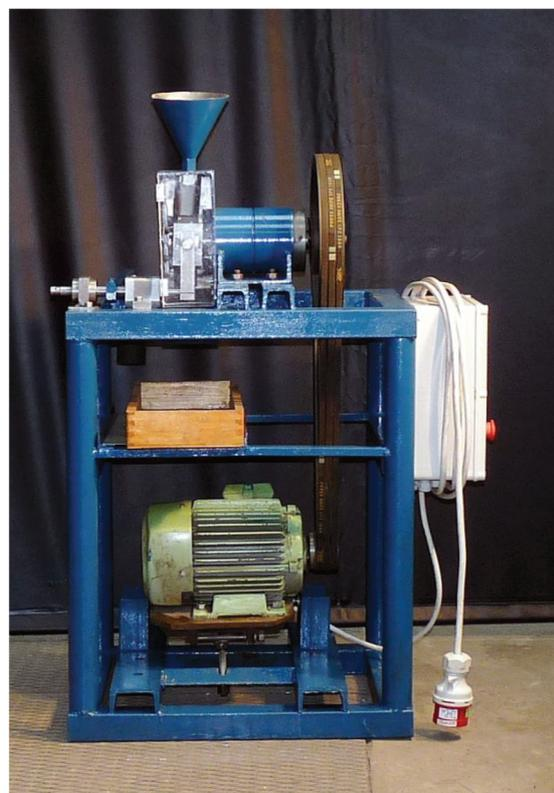
**Figure 2** Dry Sand/Rubber Wheel Apparatus for tribology testing [13]
