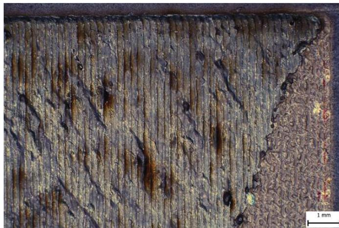
**Figure 3** High power laser trails
