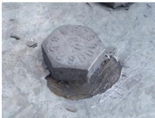
Figure 1 Example of delamination of HDG coating on construction's elements
