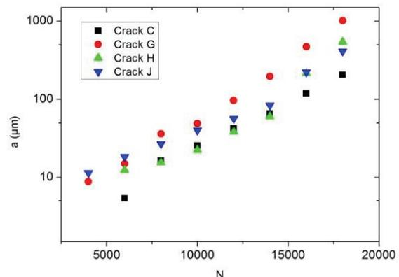
**Figure 3** An example of crack length as a function of the number of cycles. Axial tension-compression loading with strain amplitude  $\epsilon_a = 0.32\%$ .
