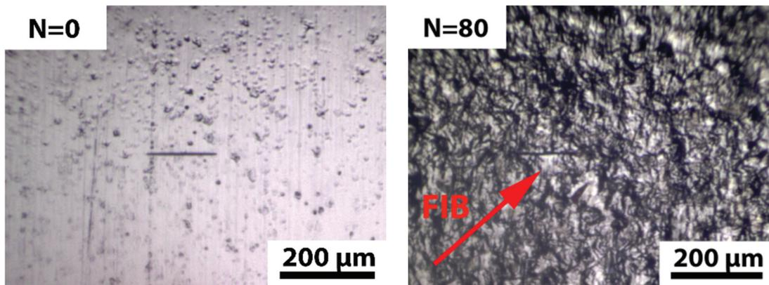
**Figure 7** Surface relief at different stages of torsional cycling. Large amount of extrusions and surface warping can be seen.
