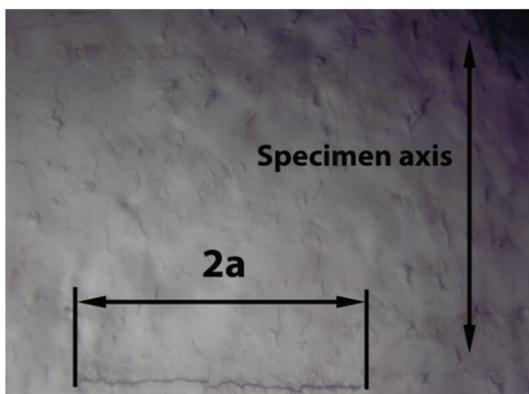
**Figure 2** Crack initiation along the slip bands in axial tension-compression loading
