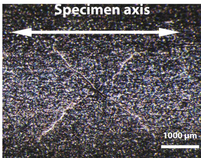
**Figure 5** Secondary crack imaged by light microscope taken after fracture in torsionally loaded sample with shear strain amplitude  $\gamma_a = 0.41\%$
