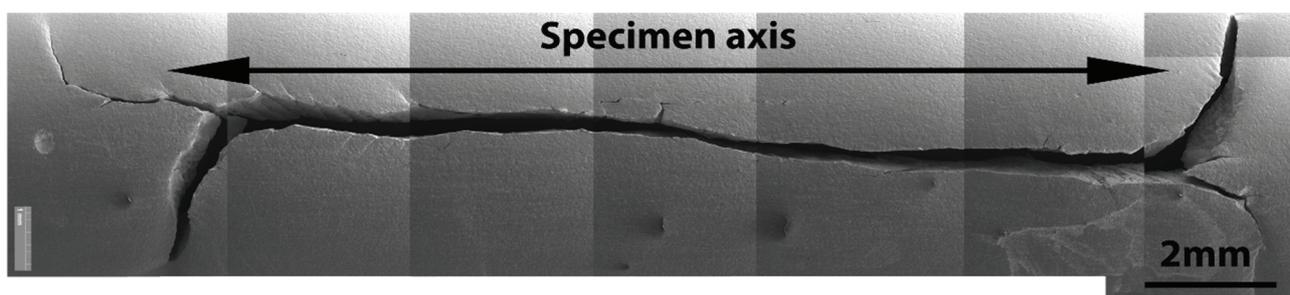
**Figure 4** SEM micrograph of specimen after fracture, loaded in torsion with shear strain amplitude  $\gamma_a = 1.732\%$ . Major crack propagating along the specimen axis direction bifurcates at the crack ends in the final stage of fatigue life.
