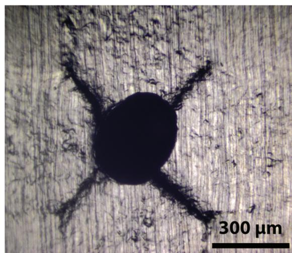
**Figure 6** Fatigue crack growth from a drilled hole after 250 fully reversed torsional cycles with a shear strain amplitude of  $\gamma_a = 0.71\%$
