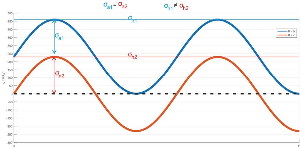
**Figure 2** Schematics of changing R ratio
