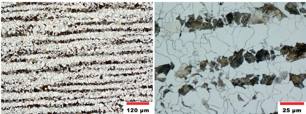
**Figure 1** Microstructure of the material S355 NL + N, left - a small magnification show well band texture, right - the detail of the microstructure
