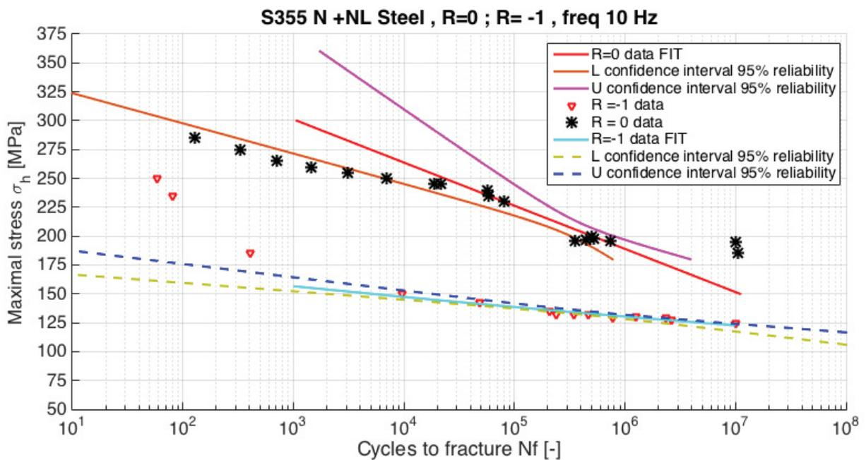
Figure 5 S-N curve, with maximal stress on Y axis, for R=0, R=-1
