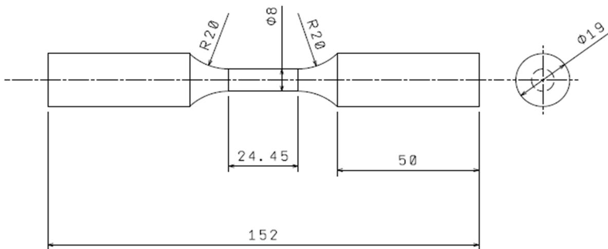
**Figure 3** Geometry of specimens
