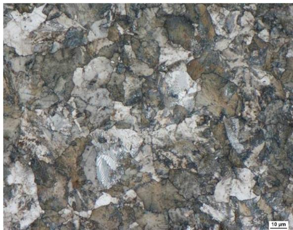
**Figure 1** Optical micrograph - initial pearlitic structure of the experimental steel
