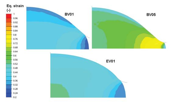
Figure 6 Shape of 1/4 section of roll stock and equivalent strain field in the output rolling plane after the first pass for the selected simulation variants
