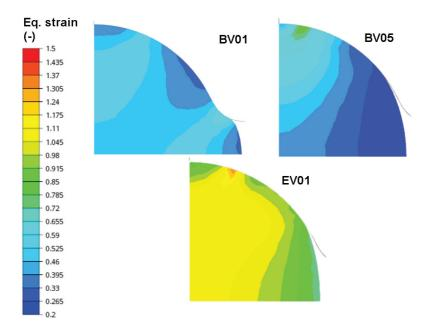
**Figure 7** Shape of 1/4 section of roll stock and equivalent strain field in the output rolling plane after the second pass for the selected simulation variants
