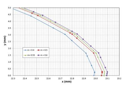
Figure 1 Effect of friction factor m on the shape of the crosssection of the stock 30 mm behind the input plane during rolling on a wane (T = 1200 °C)
