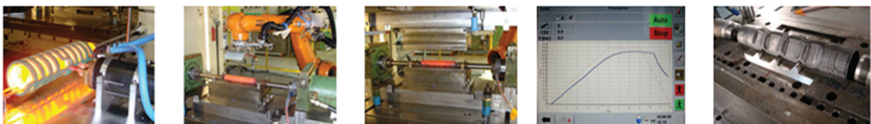
Figure 2 Process chain press hardening
