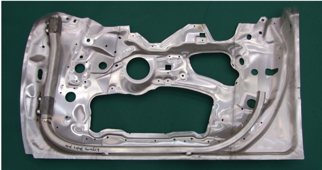
Figure 1 The inside component of a passenger car door with a joined frame
